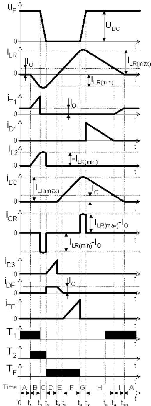
Fig. 2. Transient waveforms for the load current  $I_O > 0$
