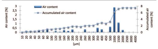
Fig. 1. The porosity characteristics of non air-entrained SCC (CEM I 32.5 R + 10% silica fume; w/b=0.41) [14].
