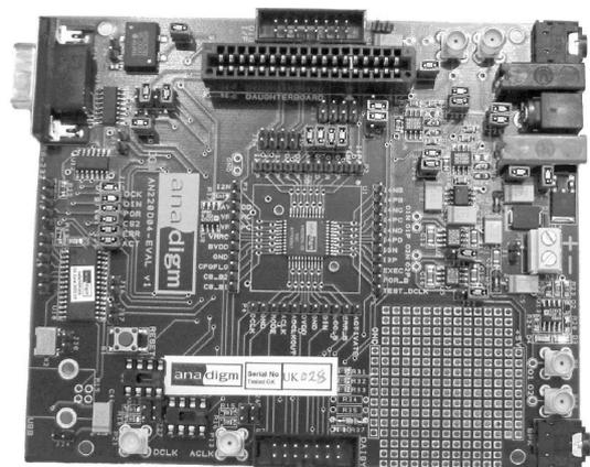
Fig. 1. Anadigm Vortex AN220D04 Evaluation Board with the AN221E04 device
