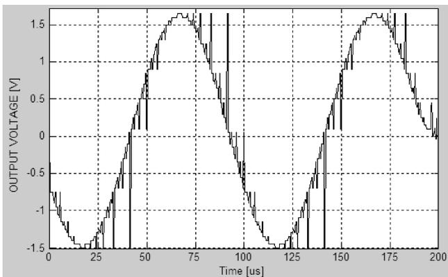
Fig. 7. Sinusoidal waveform after reconstruction digital outputs of the iterative algorithmic 6-bit ADC
