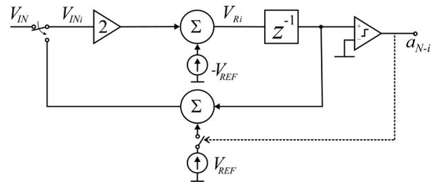
Fig. 3. Structure of an iterative algorithmic ADC
