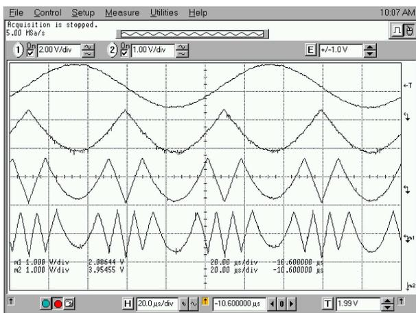
Fig. 17. Residue voltages of the Gray algorithmic 6-bit ADC
