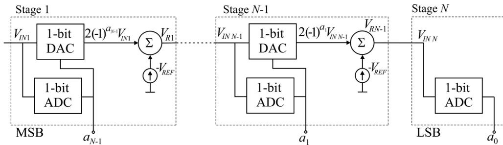
Fig. 15. Block diagram of a Gray algorithmic ADC
