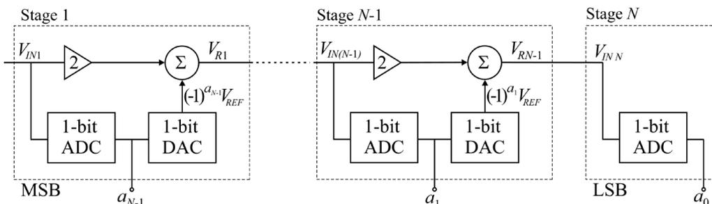
Fig. 9. Block diagram of a serial algorithmic ADC
