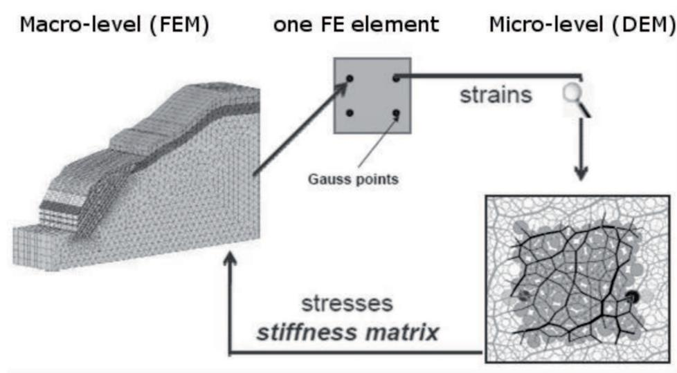
Fig. 2. Schematic representation of two-scale approach for bodies with granular micro-structure.
