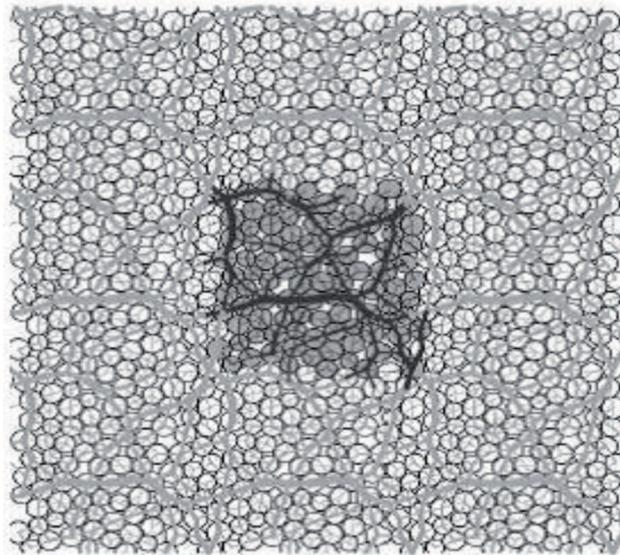
Fig. 4. Shape of periodic limit condition (PLC) specimen with normal contact forces.
