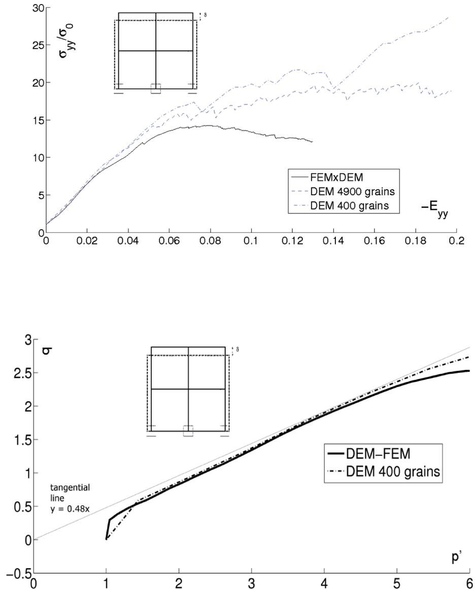
Fig. 11. Two-scale computations of biaxial test without volume changes for granular materials ( $\sigma_{yy}$  – vertical normal stress,  $\sigma_{xx}$  – horizontal normal stress,  $E_{yy}$  – vertical normal strain,  $q$  – deviatoric stress,  $p'$  – mean effective stress).
