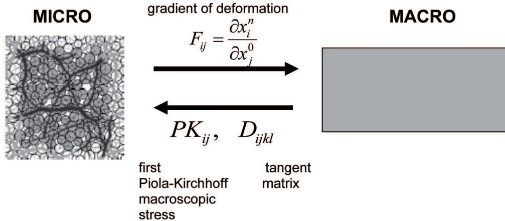
Fig. 1. Computational homogenization using discrete element method (DEM) at micro-level and finite element method (FEM) at macro-level.
