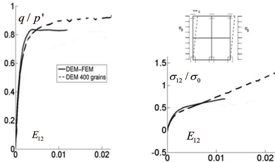
Fig. 12. Two-scale computations of shear test for granular materials ( $q$  – deviatoric stress,  $p'$  – mean effective stress,  $\sigma_{12}$  – shear stress,  $E_{12}$  – shear strain).
