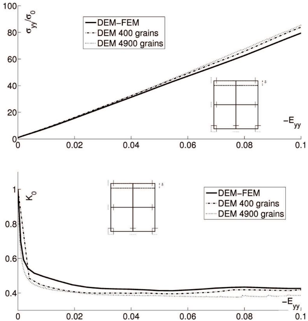
Fig. 9. Two-scale computations of oedometric test for granular materials ( $\sigma_{yy}$  – vertical normal stress,  $\sigma_{xx}$  – horizontal normal stress,  $E_{yy}$  – vertical normal strain,  $K_0 = \sigma_{xx}/\sigma_{yy}$  – the lateral earth pressure coefficient).
