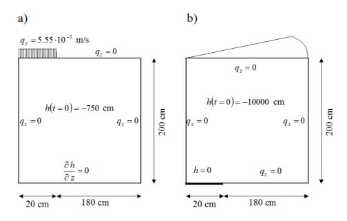
Fig. 2. Solution domain and initial and boundary conditions applied in the numerical examples: a) example 1, b) example 2.
