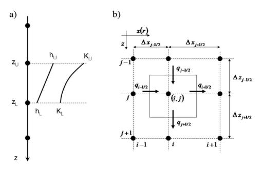
Fig. 1. Spatial discretisation of the unsaturated flow equation: a) one-dimensional in z direction, b) two-dimensional in x - z or r - z plane.
