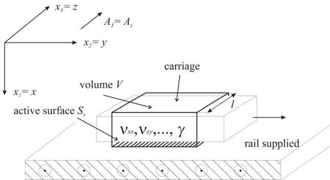
Fig. 4. Linear electromechanical converter
