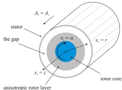
Fig. 6. Cylindrical electromechanical converter
