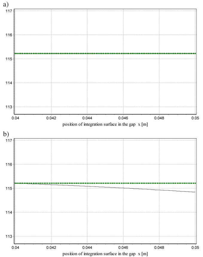
Fig. 5. Electromagnetic force vs. position of integral surface in the gap of linear motor (Maxwell and coenergy method – line Lorentz method - points)
