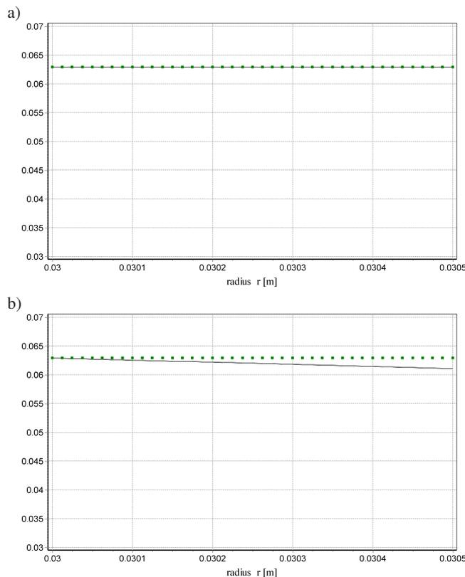
Fig. 9. Electromagnetic torque vs. radius for the gap region (Maxwell and coenergy method – line, Lorentz method – points)
