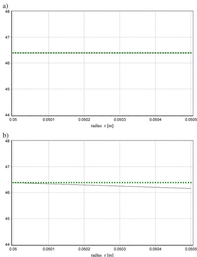
Fig. 7. Electromagnetic torque vs. radius for the gap region (Maxwell and coenergy method – line, Lorentz method – points)
