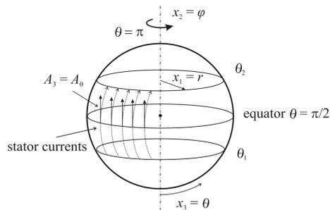
Fig. 8. Spherical electromechanical converter
