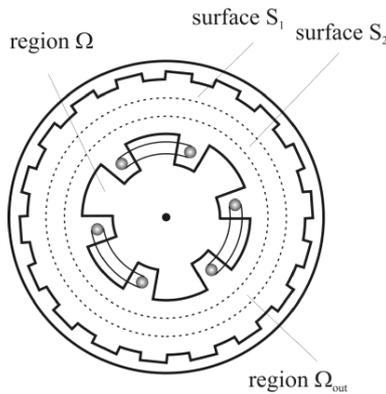
Fig. 3. The electromagnetic torque does not depend on integral-surface position in the isotropic gap
