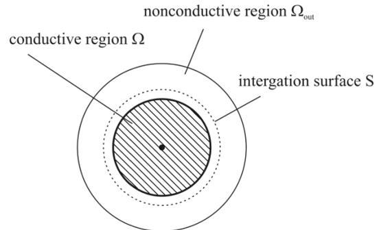
Fig. 2. The electromagnetic torque evaluation by surface integral over  $S$
