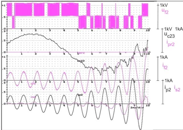
Fig. 7. Waveforms of voltages  $u_{f2}$ ,  $u_{c23}$  (1 kV/div) and currents  $i_{pr2}$ ,  $i_{f2}$ ,  $i_{p2}$ ,  $i_{s2}$  (1 kA/div) for  $R_o = 1.5 \text{ k}\Omega$ ,  $k_{up} = 0$ ,  $k_{ud} = 0$  and  $k_{id} = 0$
