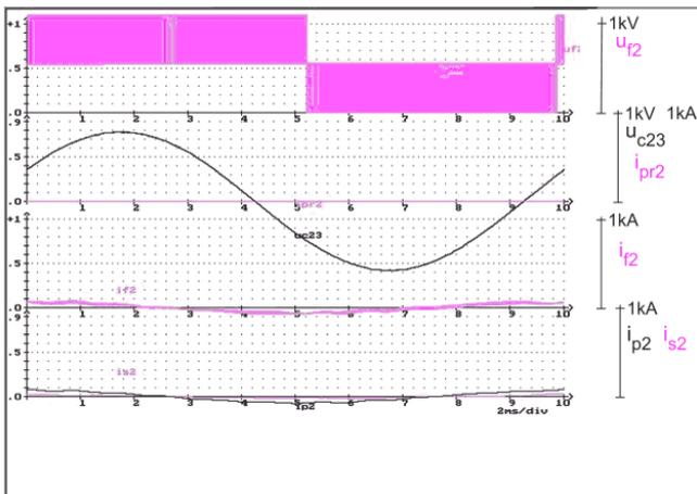
Fig. 8. Waveforms of voltages  $u_{f2}$ ,  $u_{c23}$  (1 kV/div) and currents  $i_{pr2}$ ,  $i_{f2}$ ,  $i_{p2}$ ,  $i_{s2}$  (1 kA/div) for  $R_o = 1.5 \text{ k}\Omega$ ,  $k_{up} = 0.022$ ,  $k_{ud} = 1.3 \cdot 10^{-7}$  and  $k_{id} = 8 \cdot 10^{-4}$
