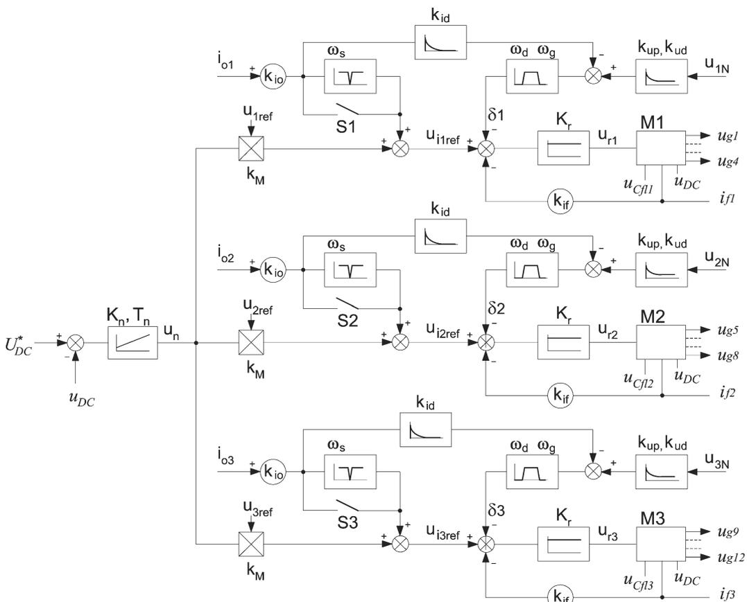
Fig. 2. Equivalent circuit of active filter control system
