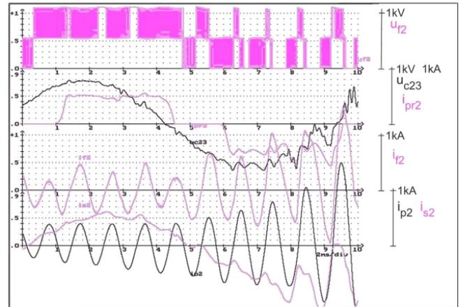
Fig. 5. Waveforms of voltages  $u_{f2}$ ,  $u_{c23}$  (1 kV/div) and currents  $i_{pr2}$ ,  $i_{f2}$ ,  $i_{p2}$ ,  $i_{s2}$  (1 kA/div) for  $R_o = 1.5$   $\Omega$ ,  $k_{up} = 0$ ,  $k_{ud} = 0$  and  $k_{id} = 0$
