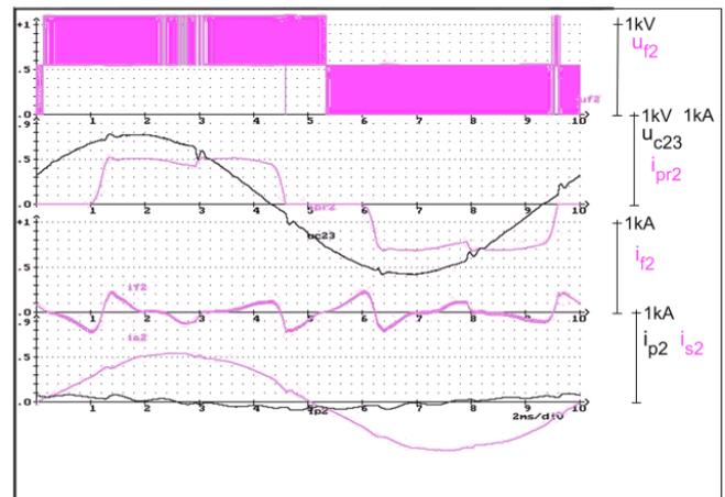
Fig. 6. Waveforms of voltages  $u_{f2}$ ,  $u_{c23}$  (1 kV/div) and currents  $i_{pr2}$ ,  $i_{f2}$ ,  $i_{p2}$ ,  $i_{s2}$  (1 kA/div) for  $R_o = 1.5$   $\Omega$ ,  $k_{up} = 0.022$ ,  $k_{ud} = 1.3 \cdot 10^{-7}$  and  $k_{id} = 8 \cdot 10^{-4}$
