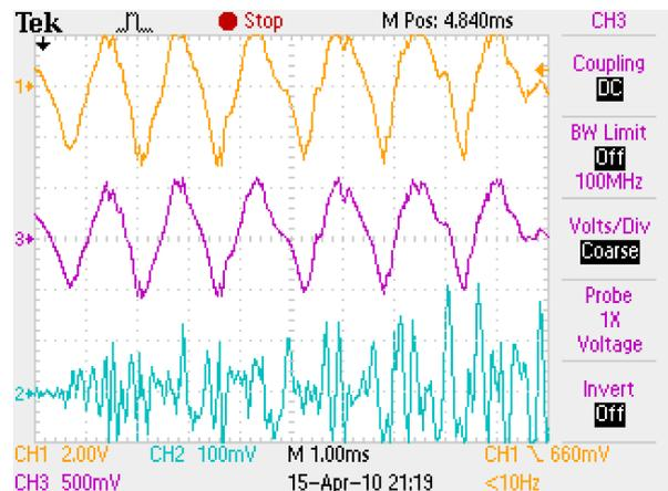
Fig. 9. Inverter output current waveform  $i_{f2}$  (CH1:400 A/div), output filter current  $i_{l2}$  (CH2:500 A/div), and capacitor  $C_{f2}$  current  $i_{cf2}$  (CH3:100 A/div) for  $k_{up} = 0$ ,  $k_{ud} = 0$ ,  $k_{id} = 0$
