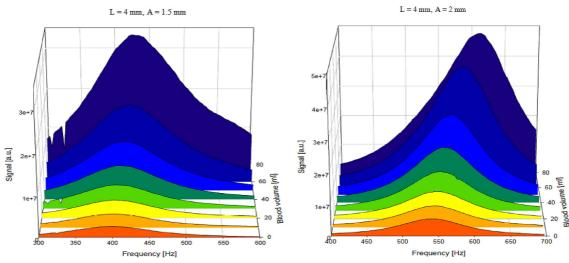
Fig. 7. Frequency characteristics of the Helmholtz resonator measurement system for different air chamber volumes
