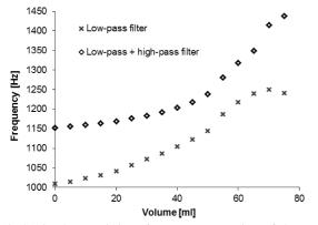
Fig. 10. Static characteristics of a new construction of the sensing system with and without the high-pass filter
