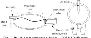
Fig. 3. Polish heart supporting device – POLVAD diagram
