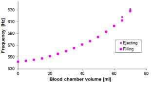
Fig. 8. Static characteristics of the acoustic sensing system
