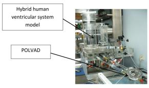
Fig. 11. Hybrid human ventricular system model for testing the POLVAD prosthesis
