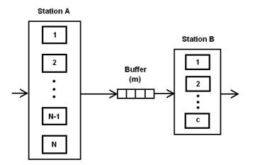
Fig. 1. Loss tandem network with blocking
