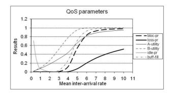
Fig. 4. Graphs of QoS parameters, where *bloc-pr* is the blocking probability, *loss-pr* is the loss probability, *A-utilization* is the station *A* utilization factor, *B-utilization* is the station *B* utilization factor, *idle-pr* is the idle probability, *buff-fill* is the buffer filling parameter
