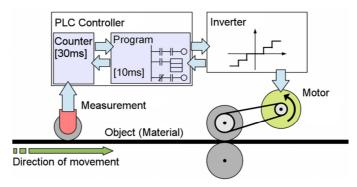
Fig. 2. Diagram of the control circuit, sampling times in brackets [8]
