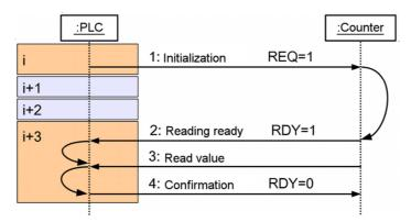
Fig. 3. Sequence diagram for the process of reading the current value of the counter [8]
