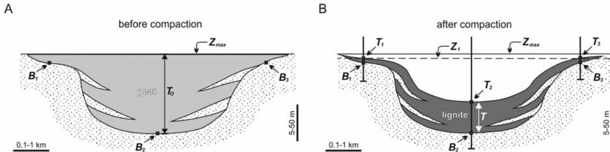
Text-fig. 8. Conceptual model of Widera's (2002) and Widera *et al.*'s (2007) method applied to estimate the compaction ratio for lignites from sedimentary basins in central Poland. Redrawn with modification from Widera (2002) and Widera *et al.* (2007)
