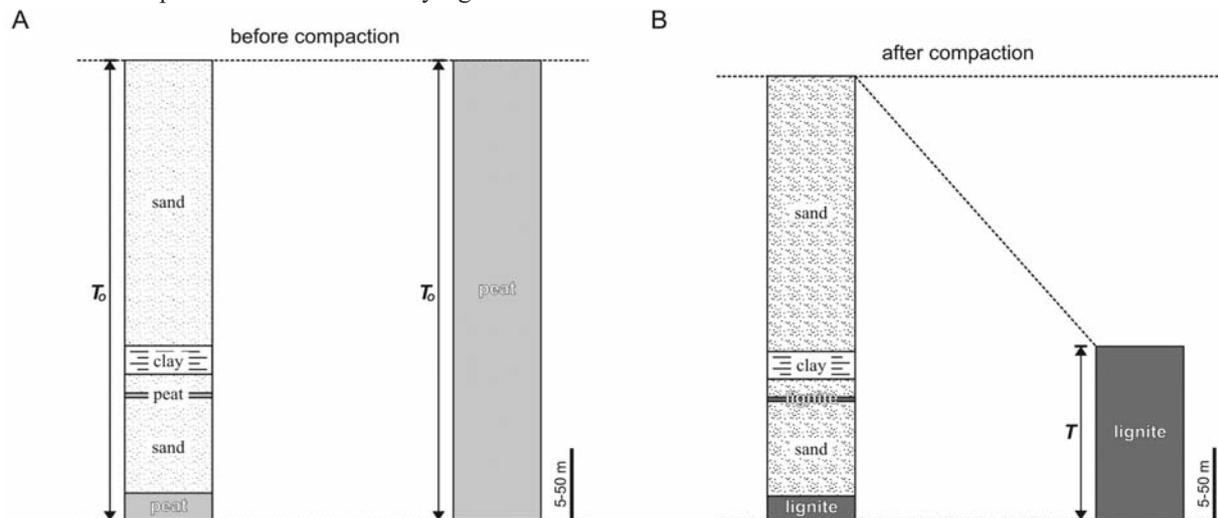
Text-fig. 7. Conceptual model of Hager *et al.*'s (1981) method applied to estimate the compaction ratio for lignites from Lower Rhine Basin in northwest Germany. Redrawn with modification from Hager *et al.* (1981) and Widera *et al.* (2007)
