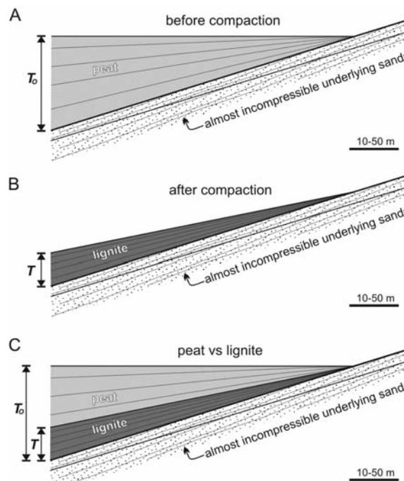
Text-fig. 6. Conceptual model of Hurník's (1972) method applied to estimate the compaction ratio for lignites from the North Bohemian Basin in the north west Czech Republic. Graphic interpretation by the author of this paper
