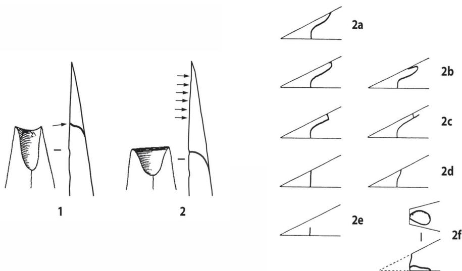
Fig. 6. Types and definitions of fractures; modified after A. Fischer et. al. (1984, 23) and M. O'Farrell (2005, p. 98).
