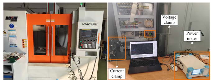
Fig. 7. VMC855H power measurement test platform
