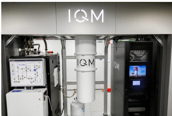
Fig. 1. Photograph of the 'ODRA-5' IQM Spark 5-qubit quantum computer installed at Wroclaw University of Science and Technology, used in our experiments
