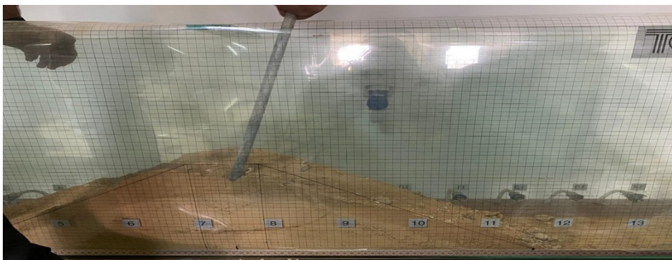
Fig. 6. Placing the soil sample in the form of layers and compacting each layer
