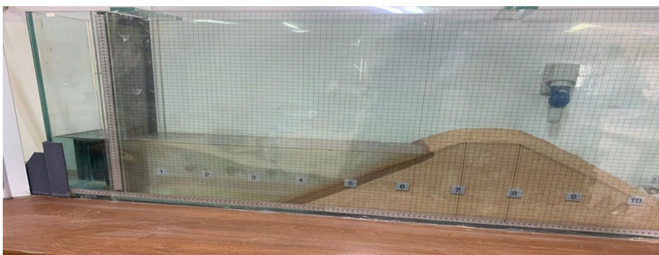
Fig. 7. Pumping water to a constant level
