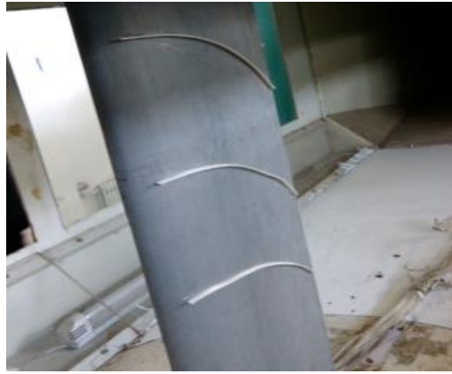
Fig.4. Experimental model of blade guide bar pressure measurement
