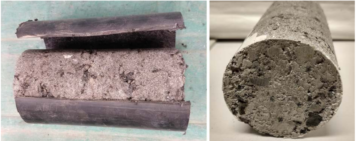
Text-fig. 2. Test sample with the plastic mould cut open (left) and basal surface of a test sample (right).
