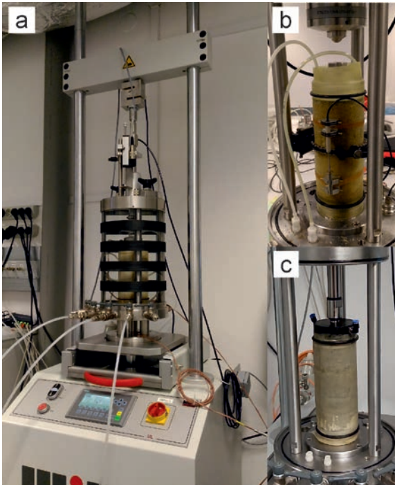
Text-fig. 4. Triaxial test setup. A – sample specimens in the triaxial cell; B – triaxial cell with local LVDT strain sensors; C – triaxial cell in basic setting.
