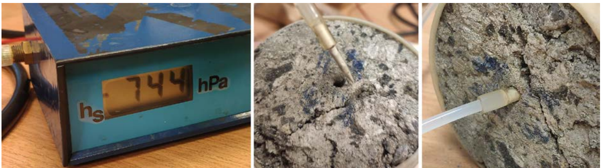
Text-fig. 5. Suction measurement: readout unit (left), ceramic needle prepared for measurement (centre), ceramic needle inserted into a prepared hole during the measurement (right).
