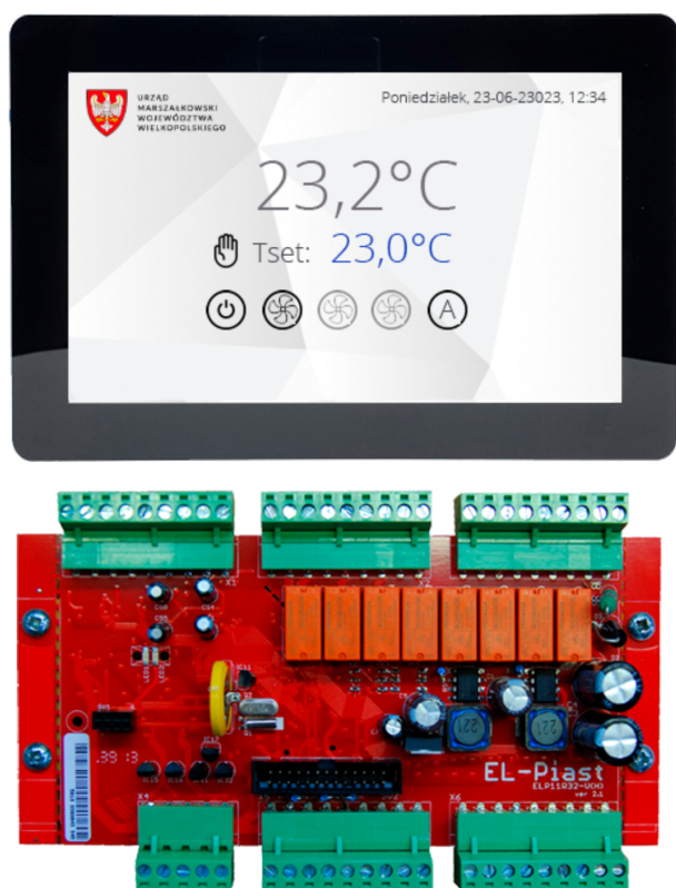
Fig. 11. A set of room automation devices designed for measuring, setting the temperature and regulating the operation of the air handling unit. The PLC controller is located in the power supply and control cabinet together with other automation components necessary for the operation of air conditioning and ventilation. The operator panel is located on the wall of the rooms
