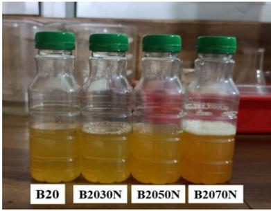
Fig. 2. Physical appearance of test fuel blends.
