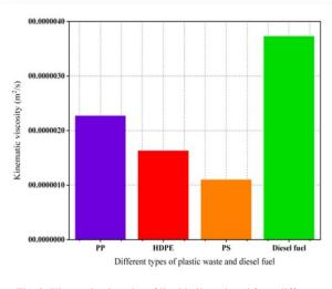
Fig. 3. Kinematic viscosity of liquid oil produced from different types of plastic waste.
