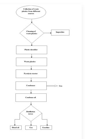
Fig. 1. Flow processes of waste plastic into oil.
