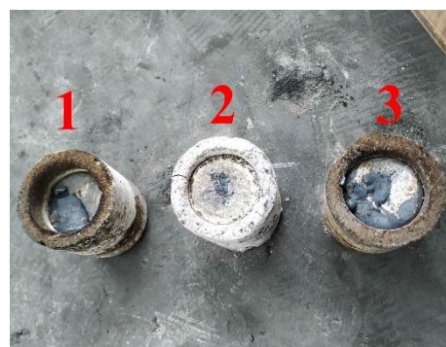
Fig. 15. Risers cut from the casting
