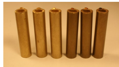
Fig. 3. Samples after the annealing process, visible burrs
