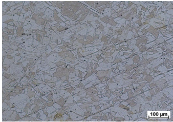
Fig. 1. Microstructure of annealed brass, magnification 100x
