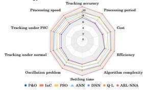
Fig. 13. Performance estimation of Al-based MPPT algorithms
