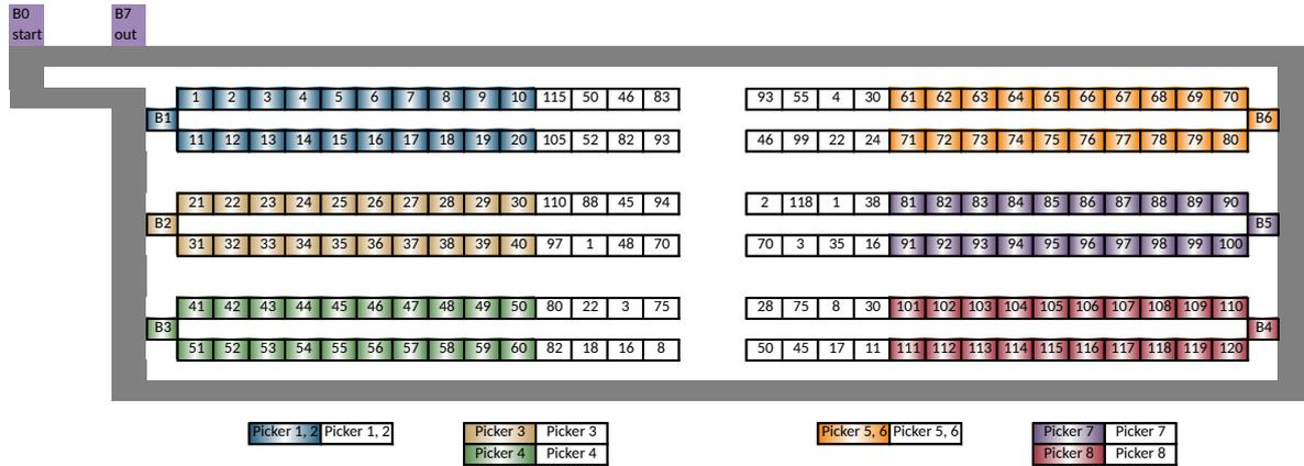
Fig. 3. The layout of a distribution center in which several pickers complete orders in one buffer: B0 – start buffer; B7 – out buffer; B1-B6 – order picking buffers; Dark colors in buffers B1-B6 – regular buffer products; Light colors in buffers B1-B6 – products also allocated in other buffers
