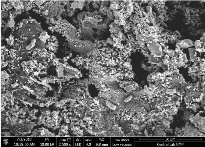
Fig. 7. Lesser Calcium Hydroxide in specimens with 10% UPOFA
