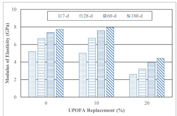
Fig. 9. Modulus of elasticity testing result
