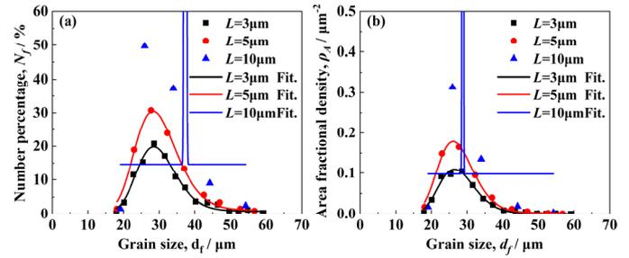
Fig. 12. The influence of interval length on the statistical accuracy of ferrite grain size at the location with  $l = 20$  mm under the fire conditions of the 700°C-120 min (a)  $N_f$ -700°C-120 min; (b)  $\rho_{Af}$ -700°C-120 min
