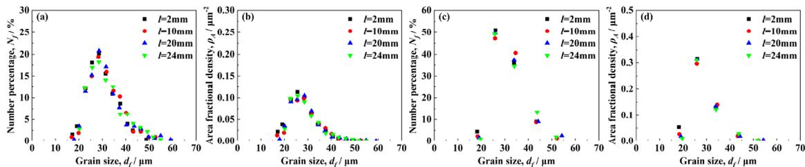
Fig. 6. Statistical results both of ferrite grain distribution parameters  $N_f$  and  $\rho_{Af}$  with two different interval lengths of 3  $\mu\text{m}$  and 10  $\mu\text{m}$  under the fire conditions of 700°C-120 min (a)  $N_f$ -700°C-120 min-3  $\mu\text{m}$ ; (b)  $\rho_{Af}$ -700°C-120 min-3  $\mu\text{m}$ ; (c)  $N_f$ -700°C-120 min-10  $\mu\text{m}$ ; (d)  $\rho_{Af}$ -700°C-120 min-10  $\mu\text{m}$
