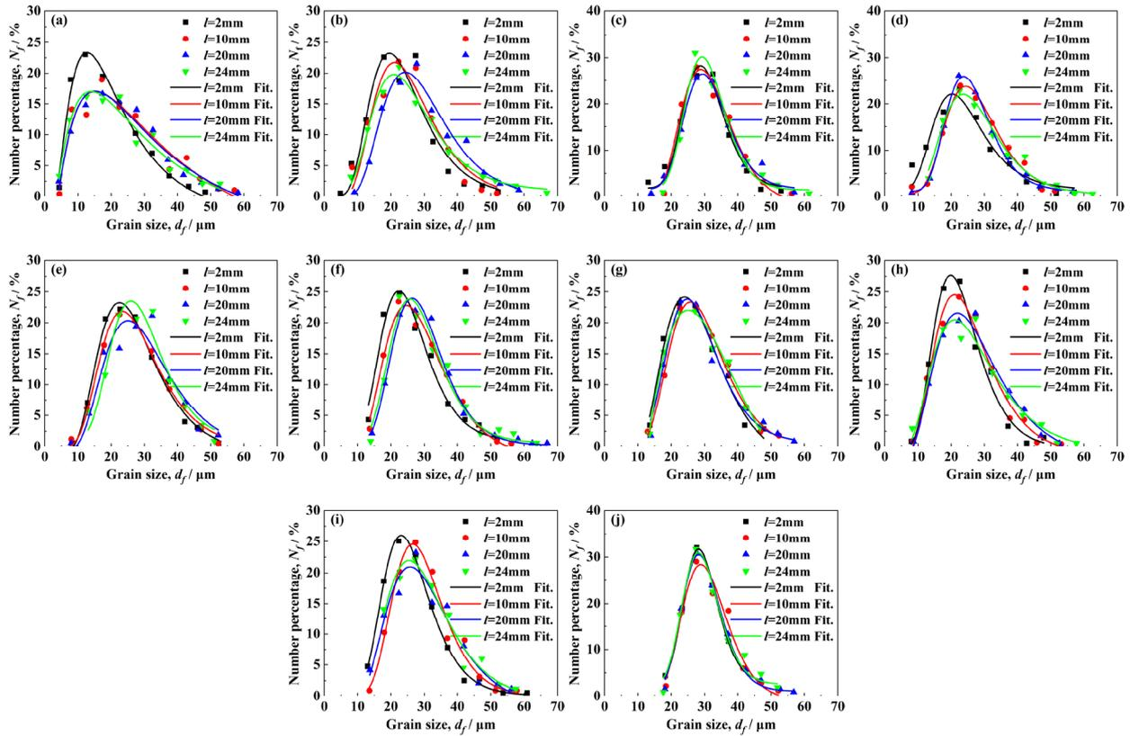
Fig. 7. The relationships between the proportion of ferrite grain number  $N_f$  and the average diameter  $d_f$  of the 40 mm-thick Q345 steel under different fire environments (a)  $N_f$ -20°C-0 min; (b)  $N_f$ -300°C-40 min; (c)  $N_f$ -500°C-40 min; (d)  $N_f$ -700°C-40 min; (e)  $N_f$ -300°C-60 min; (f)  $N_f$ -500°C-60 min; (g)  $N_f$ -700°C-60 min; (h)  $N_f$ -300°C-120 min; (i)  $N_f$ -500°C-120 min; (j)  $N_f$ -700°C-120 min
