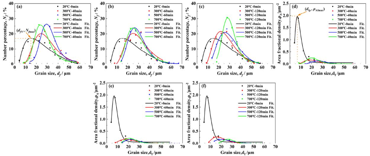
Fig. 9. The influence of fire temperature  $T$  on the non-uniform distribution of ferrite grain size in the 40 mm-thick Q345 steel (a)  $N_f$ -40 min; (b)  $N_f$ -60 min; (c)  $N_f$ -120 min; (d)  $\rho_{Af}$ -40 min; (e)  $\rho_{Af}$ -60 min; (f)  $\rho_{Af}$ -120 min
