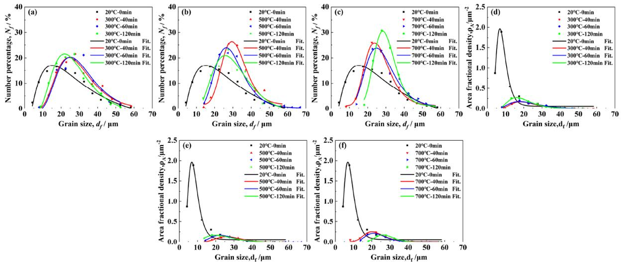
Fig. 10. The impact of fire duration on non-uniform grain distribution (a)  $N_f$ -300°C; (b)  $N_f$ -500°C; (c)  $N_f$ -700°C; (d)  $\rho_{Af}$ -300°C; (e)  $\rho_{Af}$ -500°C; (f)  $\rho_{Af}$ -700°C
