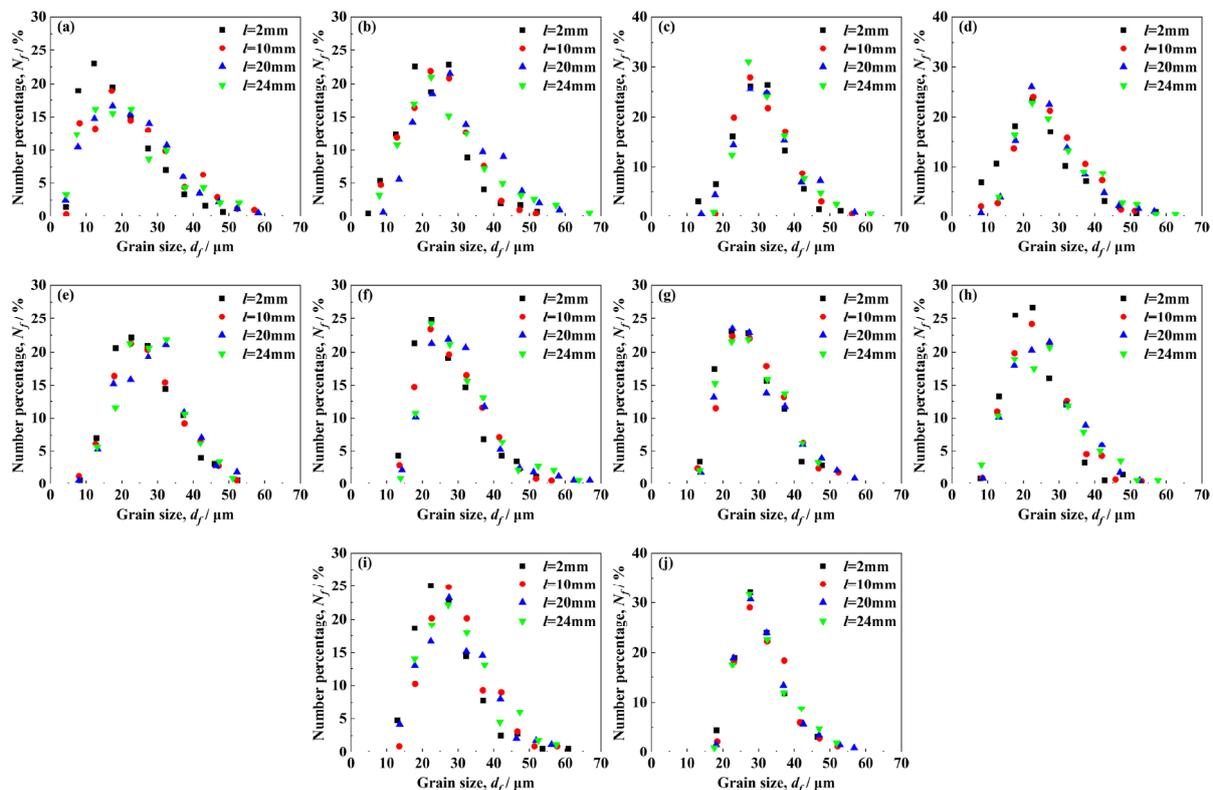
Fig. 4. Number percentage  $N_f$  of ferrite grain in the investigated 40 mm-thick Q345 steel under different fire environments (a)  $N_f$ -20°C-0 min; (b)  $N_f$ -300°C-40 min; (c)  $N_f$ -500°C-40 min; (d)  $N_f$ -700°C-40 min; (e)  $N_f$ -300°C-60 min; (f)  $N_f$ -500°C-60 min; (g)  $N_f$ -700°C-60 min; (h)  $N_f$ -300°C-120 min; (i)  $N_f$ -500°C-120 min; (j)  $N_f$ -700°C-120 min
