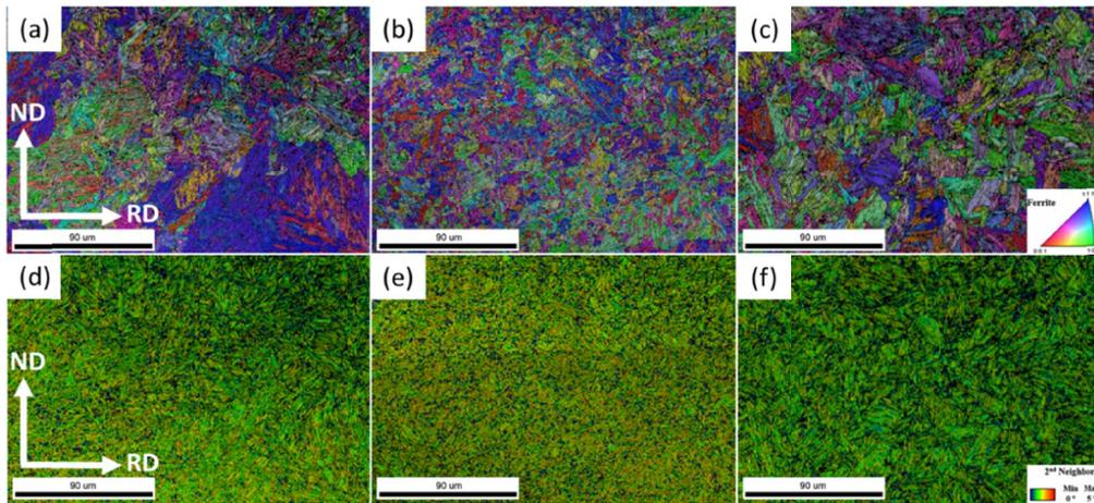
Fig. 3. Inverse pole figure (IPF) maps (a-c) and kernel average misorientation (KAM) maps (d-f) from EBSD: (a), (d) S1, (b), (e) S2, (c), (f) S3x
