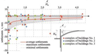
Fig.10. Results of authors' own measurements of ground settlement
