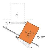
Fig.5. Impact of ground inclination T on the building structure
