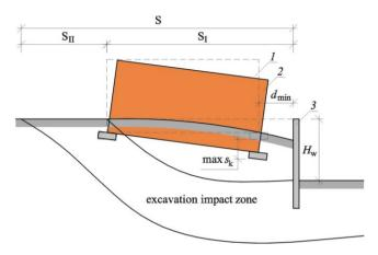
**Fig.7.** Maximum displacement of the structure acc. to [30]: 1 – state before commencement of construction works, 2 – state during construction works, 3 – support system of the excavation, S – impact area of the excavation, S<sub>I</sub> – area of direct impact of the excavation, S<sub>II</sub> – area of the secondary impact
