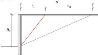
Fig.13. The area of impact zones of the excavations S<sub>I</sub> and S [30]
