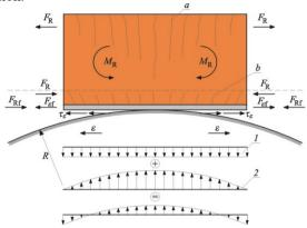
**Fig.6.** Internal forces in the building with rigid structure at the convex curvature of ground: 1 – structure foundations subjected to loading, 2 – soil reaction, 3 – load resultants acting on the building, a – cracks caused by bending, b – diagonal cracks caused by shearing and tension
