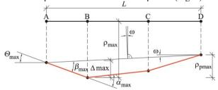
Fig.4. Symbols for the displacement of foundations acc. to EC-7 [39]
