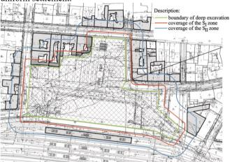
Fig.14. Impact zones of the excavation
