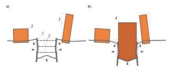
**Fig.2.** Soil displacement during different phases of performing excavation in support system: a) construction phase – performing deep excavation, b) final phase, 1 – excavation support system, 2 – elements supporting the excavation wall, 3 – nearby buildings, the constructed structure
