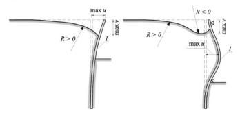
**Fig.1.** Shape of soil settlement profile within deep excavation: a) cantilever type b) spandrel type, 1 – excavation support system
