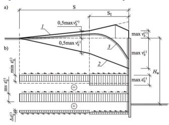
**Fig.11.** Simplified distributions of vertical displacements and deformations of the ground near the deep excavation [30]: a) vertical displacements, b) ground deformations; 1 – extreme distribution of negative displacements, 2 – extreme distribution of positive displacements, 3 – average distribution of displacements
