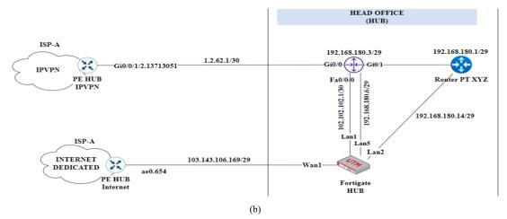
Fig. 2. LLD (Low Level Design) (a) Spoke topology (Branch Office) (b) Head office topology
