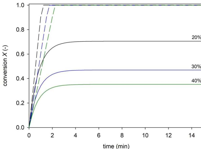
Figure 5. The conversion of starch hydrolysis by  $\alpha$ -amylase from porcine pancreas (black line – 20% starch, blue line – 30% starch, green line – 40% starch with deactivation of  $\alpha$ -amylase and dash line – without deactivation of  $\alpha$ -amylase) at 333 K in time 15 min.
