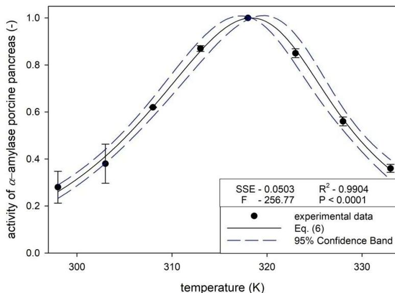
Figure 3. The effect temperature on activity of  $\alpha$ -amylase from porcine pancreas with starch hydrolysis for 15 min.
