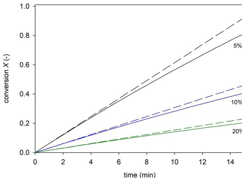
Figure 4. The conversion of starch hydrolysis by  $\alpha$ -amylase from porcine pancreas (black line – 5% starch, blue line – 10% starch, green line – 20% starch with deactivation of  $\alpha$ -amylase and dash line – without deactivation of  $\alpha$ -amylase) at 310 K for 15 min.
