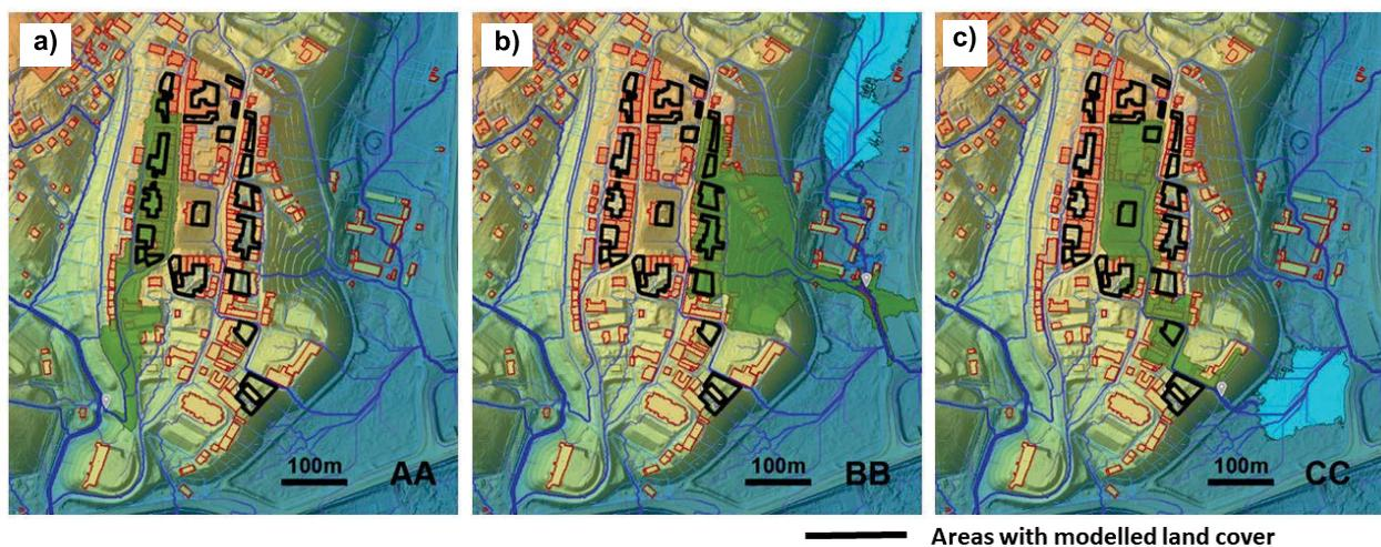
**Fig. 3.** Three (sub)runoff areas (as green markings) during modelling – scenario III, which determine the surface runoff amount and the range for the studied spaces: a) AA, b) BB, c) CC; source: own elaboration based on SCALGO Live Poland
