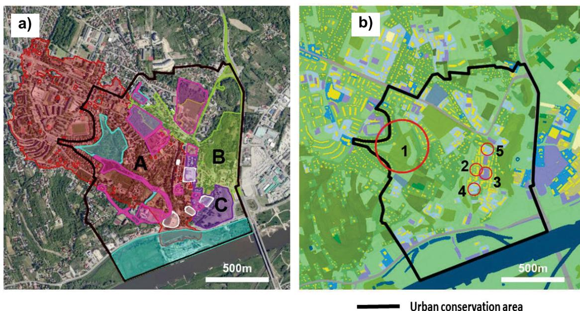
**Fig. 2.** Research scope within the city of Sandomierz: a) three main runoff areas A, B, C (chosen and named clockwise) overlapped with protected areas (compare with Fig. 1), b) selection of case studies for calculating and modelling of biologically active area on land cover layer: 1 = Piszczele Park, 2 = tenement houses courtyard in the old town, 3 = Old Town Square, 4 = town hall, 5 = St. Spirit hospital; source: own elaboration based on SCALGO Live Poland
