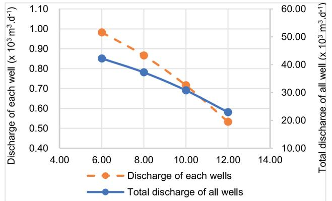
Fig. 5. The relationship between  $h_{limit}$  and maximum pumping flow rate in case 1; source: own study
