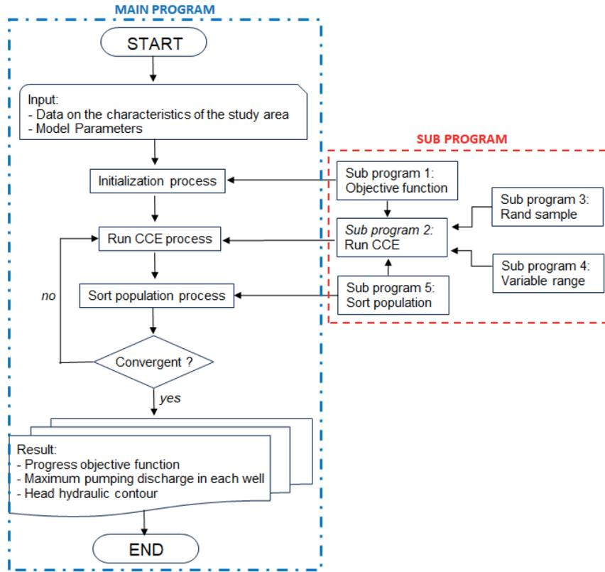
Fig. 3. The structure of the application program involves the groundwater management optimisation model based on the shuffled complex evolution (SCE-UA) algorithm; source: own study
