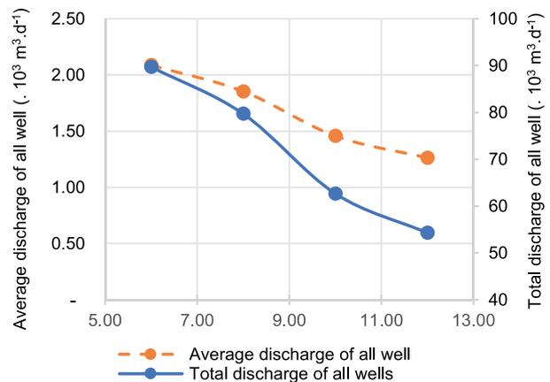
**Fig. 8.** Relationship between  $h_{limit}$  and maximum pumping rate in case 2; source: own study
