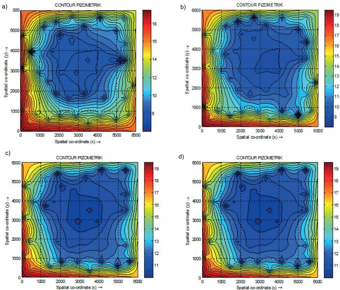
Fig. 10. Contour hydraulic head at optimum conditions in case 2: a) scenario 1, b) scenario 2, c) scenario 3, d) scenario 4; source: own study
