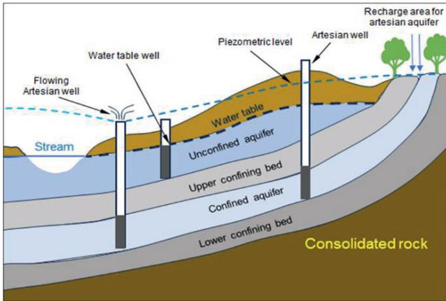
Fig. 1. Aquifer structure in soil layer; source: own elaboration
