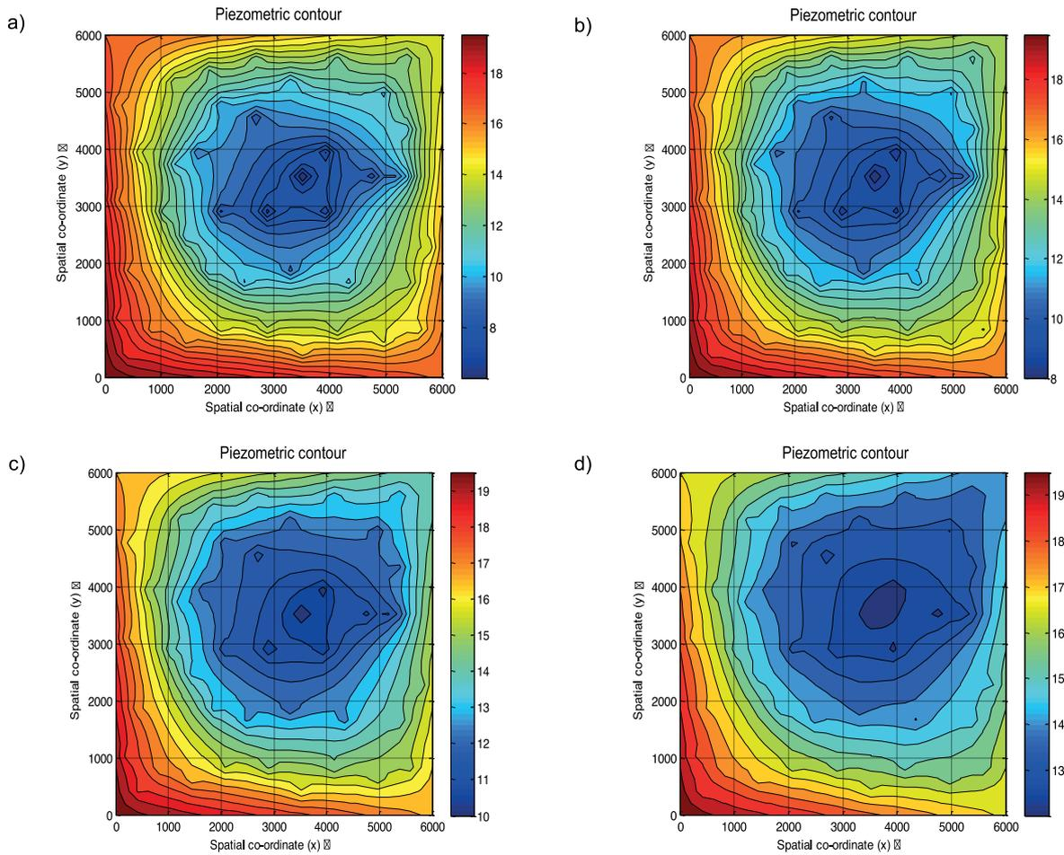
**Fig. 6.** Contour hydraulic head at optimum conditions in case 1: a) scenario 1, b) scenario 2, c) scenario 3, d) scenario 4; source: own study
