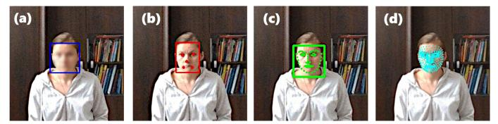
Fig. 1. Face detection models as (a) a bounding box with a face, (b) a bounding box with a face and its five points, (c) a bounding box and 68 facial points (d) 468 facial points
