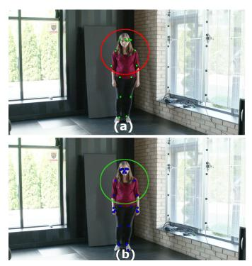
Fig. 11. Comparison of pose detection precision by (a) the MoveNet Thunder model with (b) the BlazePose model
