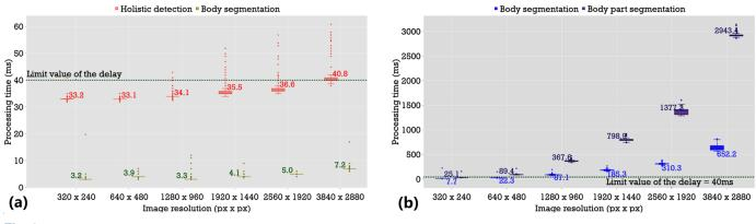
Fig. 9. Processing time for a) holistic detection and body segmentation from MediaPipe library, b) body and body part segmentation available in tfbodypix python package
