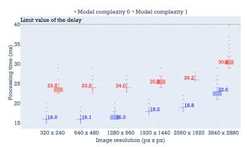
Fig. 8. Processing time for the two BlazePose models depending on the resolution of the input image
