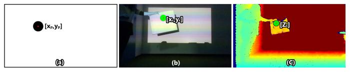
Fig. 5. The calibration process a) the image with one circle displayed by a projector, b) circle detection in the RGB image, c) reading the corresponding depth value of the circle centre on the depth map
