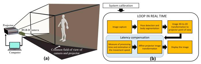
Fig. 6. (a) Dynamic lighting system, (b) diagram of the dynamic lighting process of a moving figure
