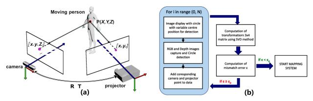
Fig. 4. (a) The point transformation from the camera to the projector layout, system. (b) diagram of the calibration process of the camera-projector
