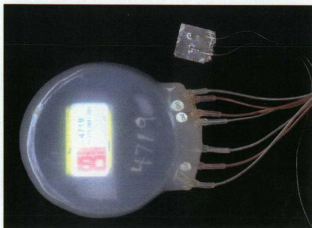
**This telemetric implant with bipolar electrodes of our own design, implanted in piglets, collects data about intestinal contractile activity**
