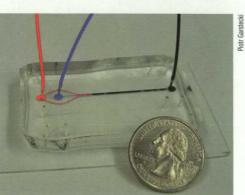
A microfluidic flow-focusing device
