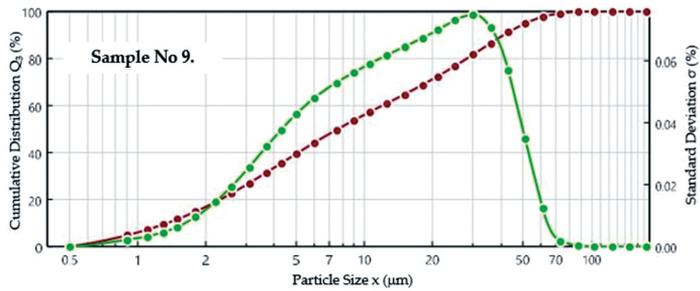
Fig. 11. The cumulative particle size distribution with standard deviation for sample No. 9
