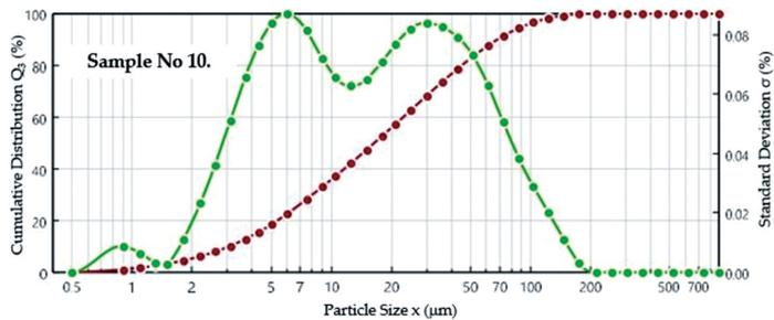
Fig. 12. The cumulative particle size distribution with standard deviation for sample No. 10
