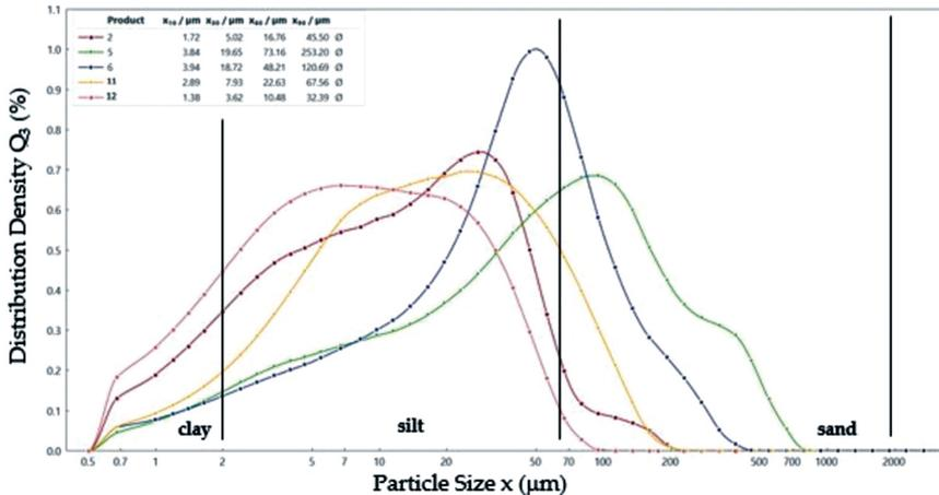
Fig. 20. The particle size Distribution Density for high-organic soils
