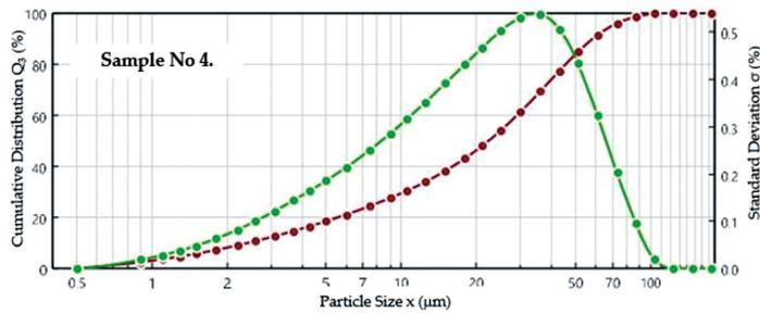
Fig. 6. The cumulative particle size distribution with standard deviation for sample No. 4
