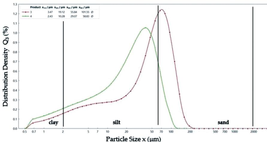
Fig. 18. The particle size Distribution Density for low-organic soils
