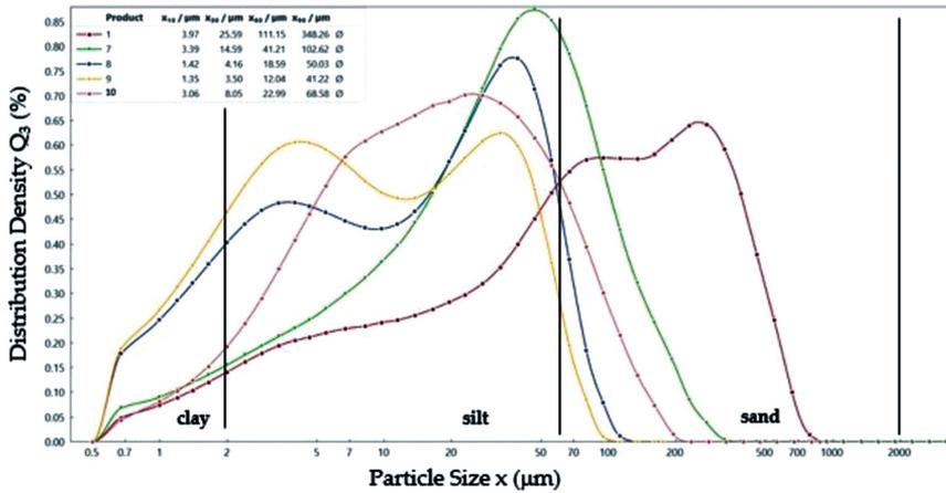
Fig. 19. The particle size Distribution Density for medium-organic soils
