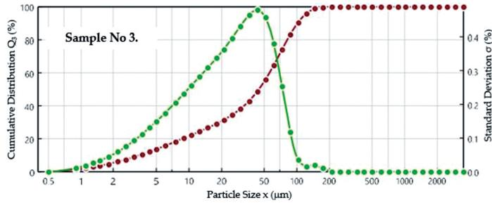
Fig. 5. The cumulative particle size distribution with standard deviation for sample No. 3
