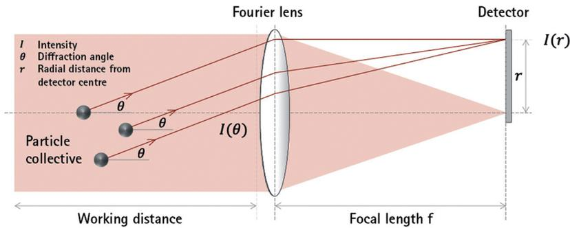
Fig. 2. The Laser Diffraction with parallel laser beam and large working zone [33]
