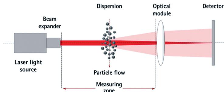
Optical setup | ISO 13320, § 5, fig. 2 for particle size from 0.1  $\mu\text{m}$  to approx. 3.0 mm
