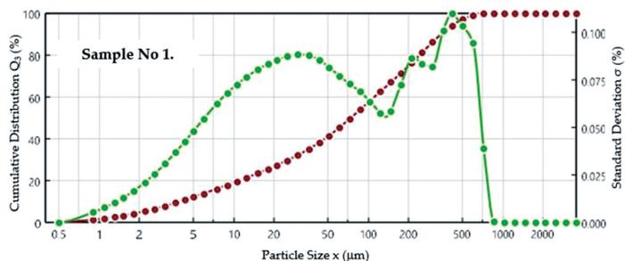
Fig. 3. The cumulative particle size distribution with standard deviation for sample No. 1
