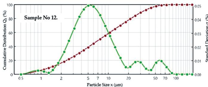
Fig. 14. The cumulative particle size distribution with standard deviation for sample No. 12
