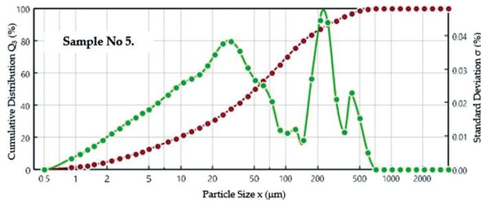
Fig. 7. The cumulative particle size distribution with standard deviation for sample No. 5
