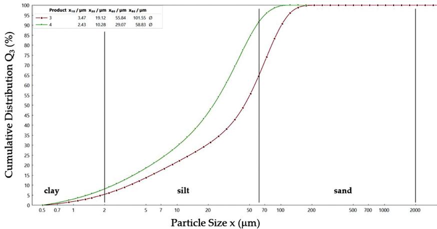
Fig. 15. The particle size cumulative distribution density for low-organic soils (sample No. 3, 4)
