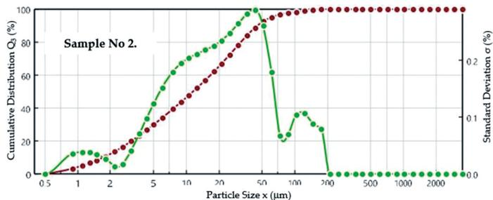
Fig. 4. The cumulative particle size distribution with standard deviation for sample No. 2
