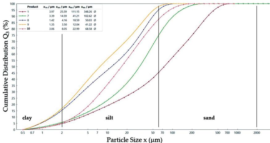
Fig. 16. The particle size cumulative distribution density for medium-organic soils (sample No. 1, 7–10)
