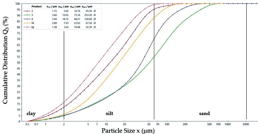
Fig. 17. The particle size cumulative distribution density for high-organic soils (sample No. 2, 5, 6, 11, 12)
