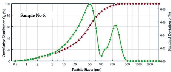
Fig. 8. The cumulative particle size distribution with standard deviation for sample No. 6
