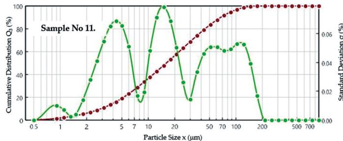
Fig. 13. The cumulative particle size distribution with standard deviation for sample No. 11
