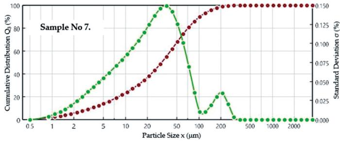
Fig. 9. The cumulative particle size distribution with standard deviation for sample No. 7
