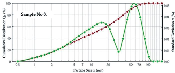
Fig. 10. The cumulative particle size distribution with standard deviation for sample No. 8
