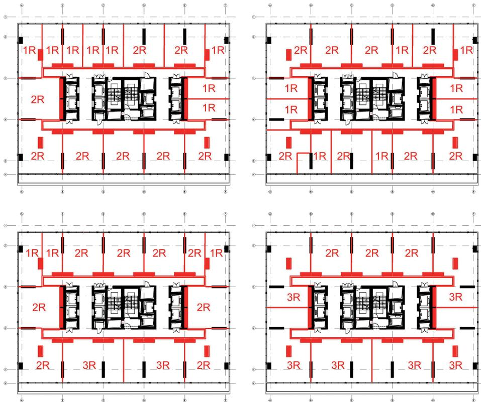
Fig. 6. Examples of variants of the setup of types of apartments on the tower floor. Other combinations of mixing of apartment types on floors were also possible. No of rooms marked on the layout; source: Author's study
