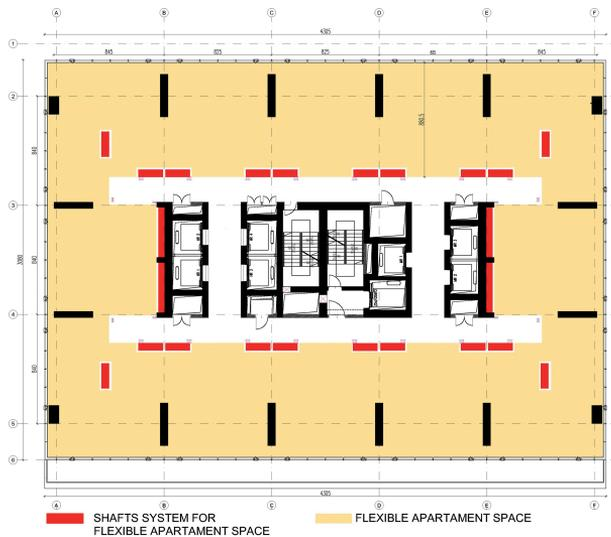
Fig. 4. The layout of the tower portion indicating hard and soft elements and systems;
