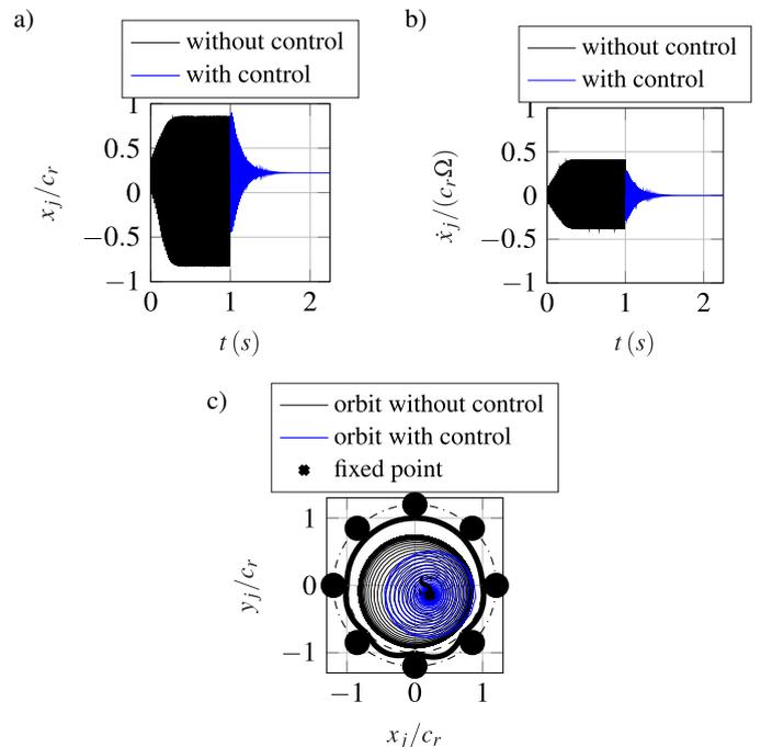
**Fig. 6.** Open and closed loop a)  $x$ -displacement, b) velocity, and c) orbit of the center of the disc at  $\Omega = 850$  rad/s. Linear control, bearing D100, disc mass  $m_d = 1$  kg, balanced rotor
