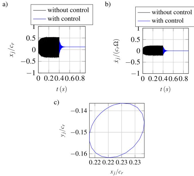
**Fig. 7.** Open and closed loop a)  $x$ -displacement, b) velocity, and c) orbit of the center of the disc at  $\Omega = 1550$  rad/s. Linear control, bearing D30, disc mass  $m_d = 0.1$  kg, balanced rotor
