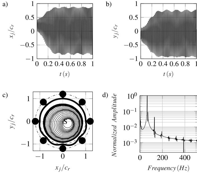
**Fig. 5.** a)  $x$ -displacement, b)  $y$ -displacement, c) orbit, and d)  $x$ -displacement signal representation in the frequency domain of the centre of the disc at  $\Omega = 850$  rad/s. Bearing D100, disc mass  $m_d = 1$  kg, foil thickness  $h_f = 0.5$  mm, unbalance grade G6.3
