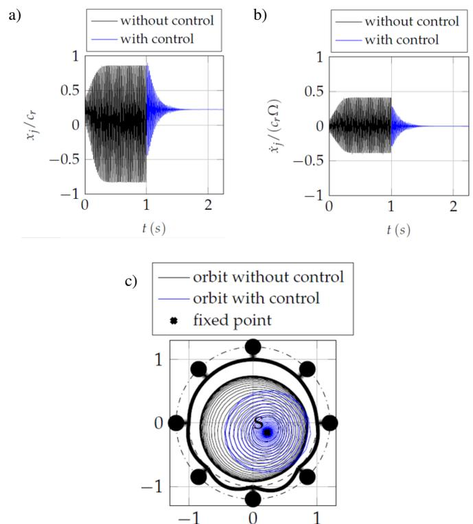
**Fig. 8.** Open- and closed-loop a)  $x$ -displacement, b) velocity, and c) orbit of the center of the disc at  $\Omega = 850$  rad/s. Polynomial feedback control, bearing D100, disc mass  $m_d = 1$  kg, balanced rotor
