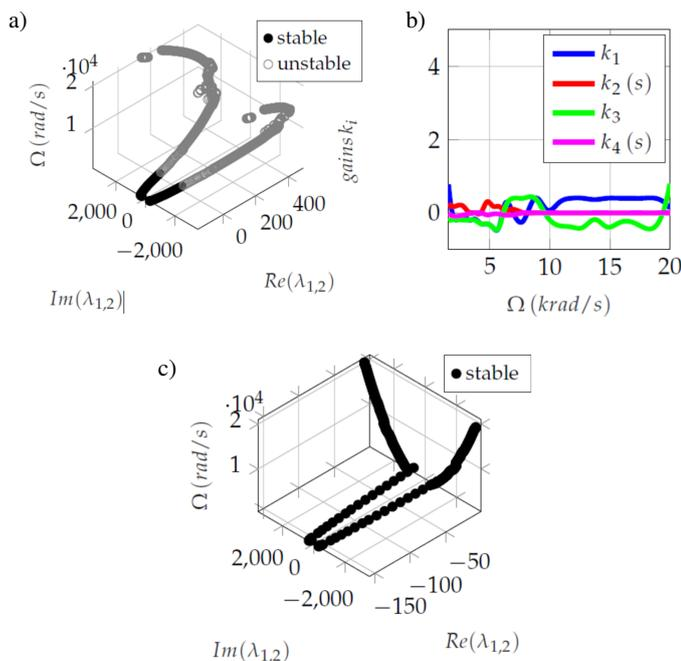
**Fig. 10.** a) open loop dominant eigenvalues, b) feedback gains for every value of the rotational speed with initially unstable fixed point, and c) close loop dominant eigenvalues
