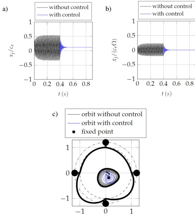
**Fig. 9.** Open and close loop a)  $x$ -displacement, b) velocity, and c) orbit of the center of the disc at  $\Omega = 850$  rad/s. Polynomial feedback control, bearing D100, disc mass  $m_d = 1$  kg, unbalance grade G6.3
