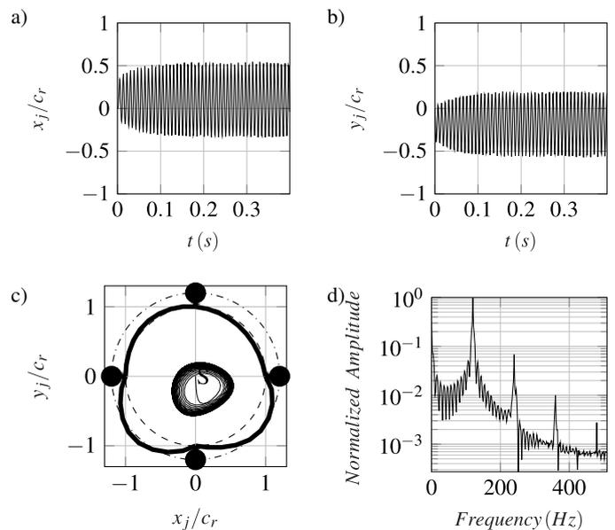
**Fig. 4.** a)  $x$ -displacement, b)  $y$ -displacement, c) orbit, and d)  $x$ -displacement signal representation in the frequency domain of the centre of the disc at  $\Omega = 1550$  rad/s. Bearing D30, disc mass  $m_d = 0.1$  kg, foil thickness  $h_f = 0.1$  mm, unbalance grade G2.5
