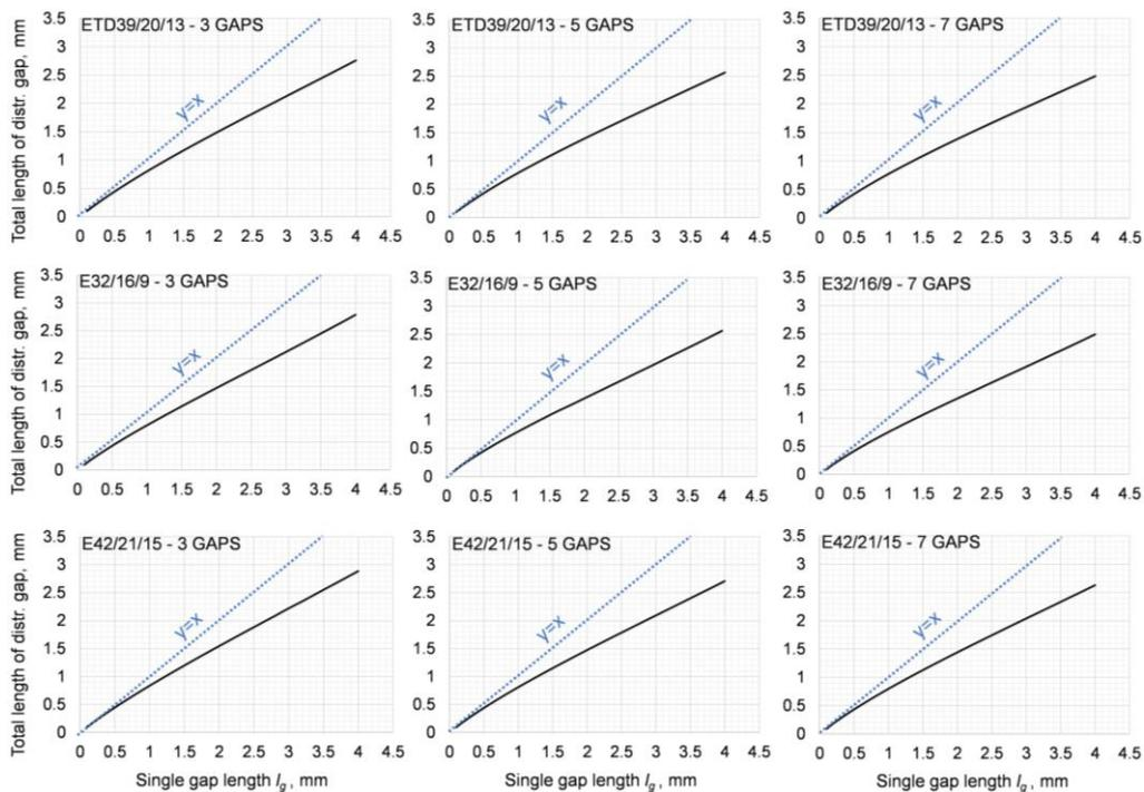
Fig. 12. Single-gap lengths and corresponding quasi-distributed-gap lengths that result in the same  $L$  if incorporated in magnetic components featuring ETD39/20/13, E32/16/9 and E42/21/15 type cores
