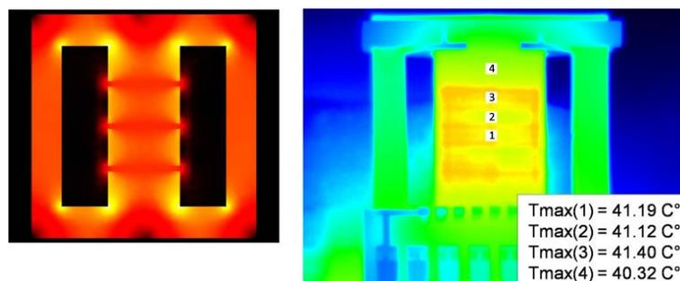
Fig. 3. Left, magnetic field density distribution in inductor with multi-gapped core (thermal scale – COMSOL® 5.2a); right, thermal image of inductor with quasi-distributed air gap
