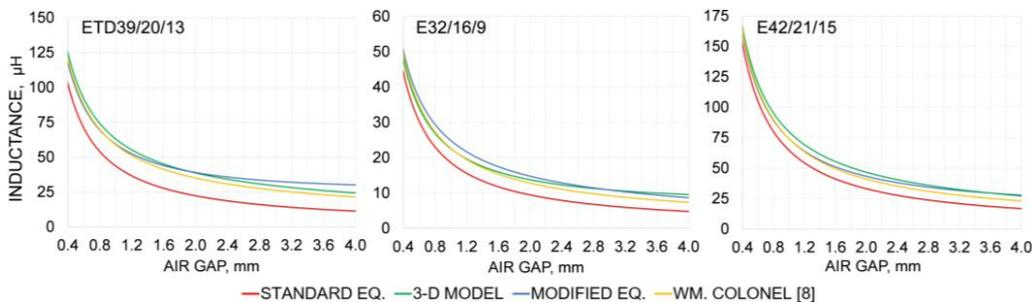
Fig. 8. Inductance values yielded by standard equation (red), 3-D model (green), modified equation (blue), and equation given in [8] for ETD, E32, and E42 type cores
