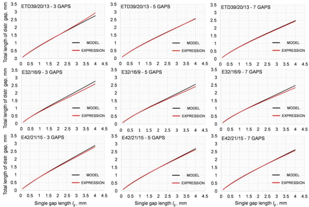
Fig. 14. Single-gap lengths and corresponding total quasi-distributed-gap lengths (red – formulae, black – FEM computations) that result in the same  $L$  if incorporated in magnetic components featuring ETD39/20/13, E32/16/9 and E42/21/15 type cores
