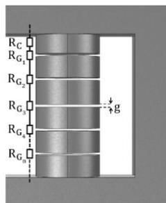
Fig. 13. Reluctance of magnetic core with quasi-distributed air gap
