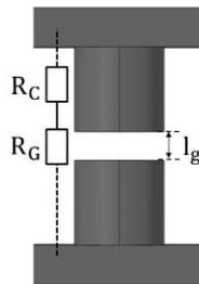
Fig. 6. Reluctance of magnetic core with single air gap
