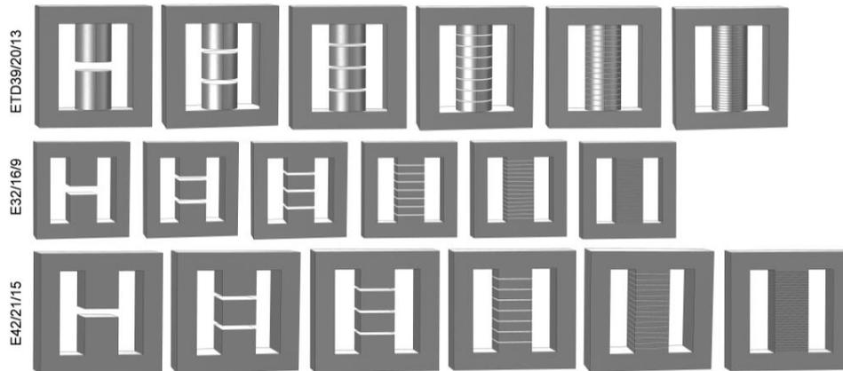
Fig. 9. Modelled cores configurations: single gap, double gap, three gaps, seven gaps, fifteen gaps and thirty-one gaps, all with total length of 3.0 mm. (Top) ETD39/20/13, (middle) E32/16/9, (bottom) E42/21/15
