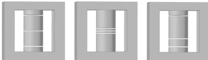
Fig. 5. Magnetic cores of the same material and total air-gap length, yielding different values of inductance for identical coils
