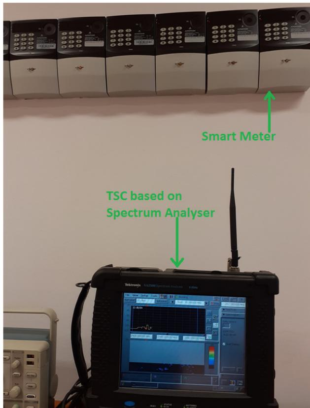
Fig. 4. Fragment of the testbed installation
