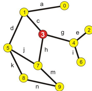
**Fig. 2.** Optimal last mile network topology with the data concentrator in the smart meter number 3
