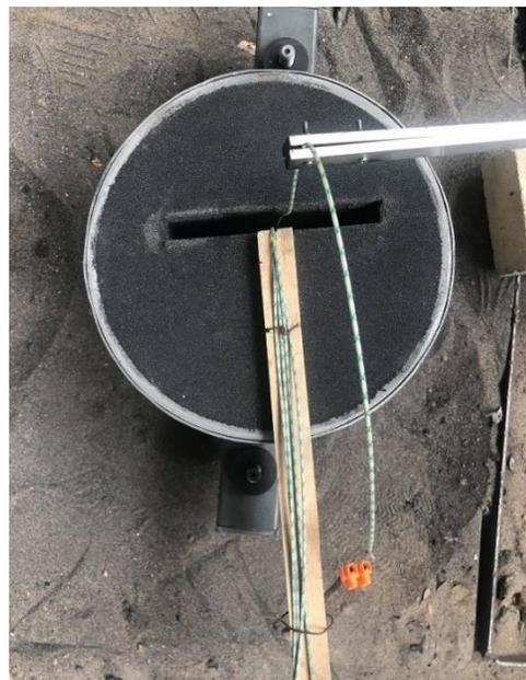
Fig. 3. Method of mounting Pt-PtRh10 thermocouples in the form. The experimental mould with visible thermocouples mounted in the mould
