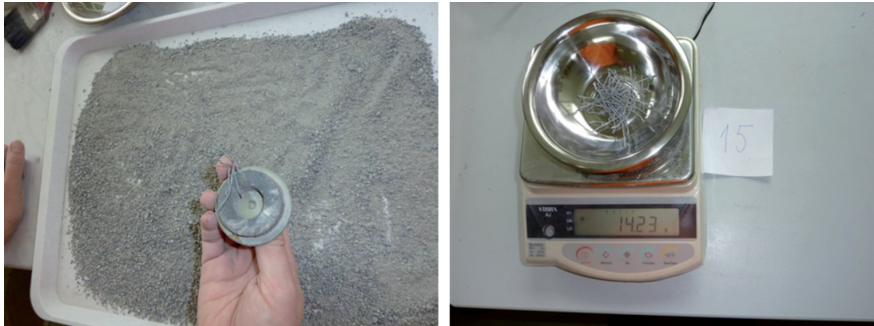
Fig. 6. Determination of the number of fibers in individual samples (Industrial floor of the production hall in Ostrava–Vítkovice)
