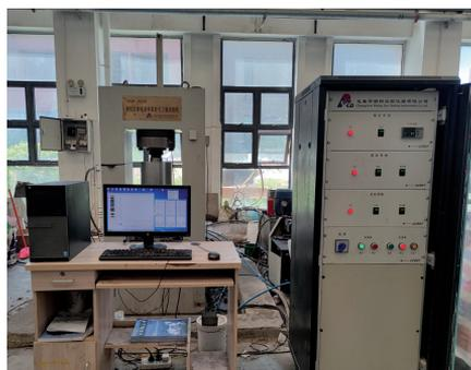
Fig. 2. TAW-2000 rock servo test system
