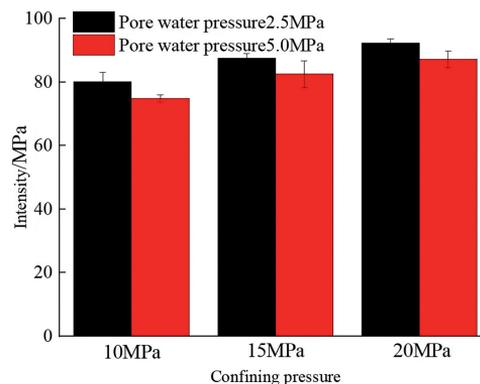
Fig. 4. Failure strength of chlorite schist in triaxial compression permeability state
