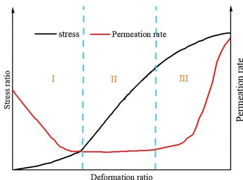
Fig. 6. Permeability evolution model of chlorite schist
