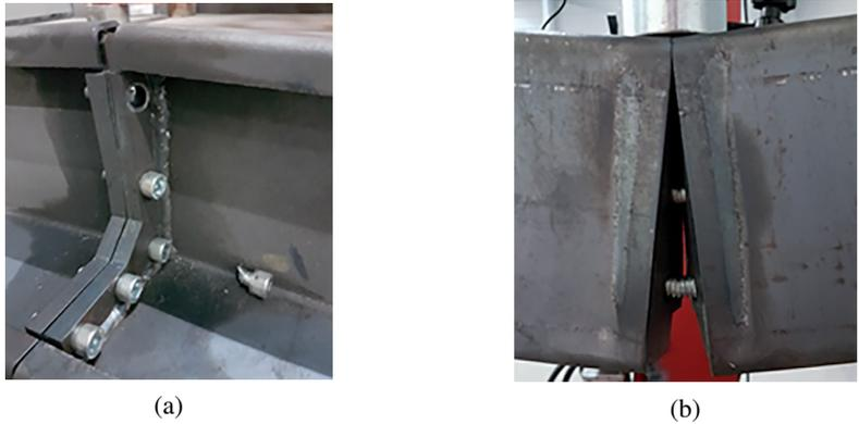
Fig. 17. Samples of the type 3.1 joint: (a) failure due to the plasticization of the material and the breaking of the most outer bolt, (b) the opening of the joint plates after failure
