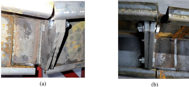
Fig. 8. Samples of the type 1 joint: (a) failure due to plasticization of the plates and the braking of the most outer bolt, (b) plasticization of the plates and the most outer bolt
