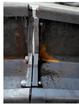
Fig. 11. Samples of the type 2.1 joint: (a) failure due to plasticization of the plates and the breaking of the thread of the most outer bolt, (b) opening of the joint plates after failure
