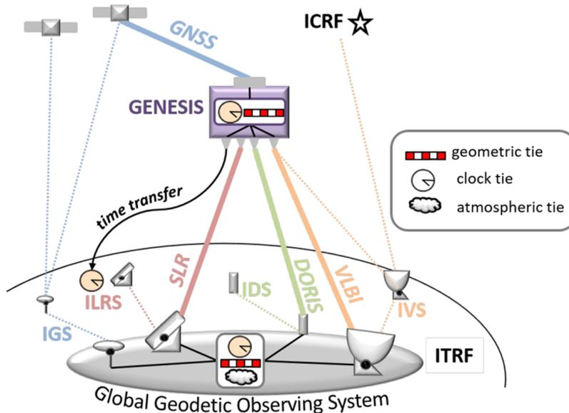
Fig. 3. Concept of the GENESIS mission for the SLR, GNSS, DORIS, and VLBI co-location in space, after Delva et al. (2023)
