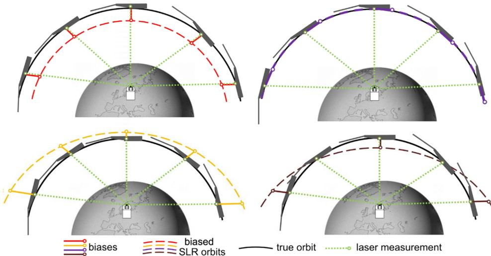
Fig. 7. Geometry of systematic errors in SLR. Range bias (top-left, red), time bias (top-right, purple), tropospheric bias (bottom-left, yellow), and sum of errors (bottom-right, brown), after Otsubo et al. (2019) and Strugarek et al. (2022)
