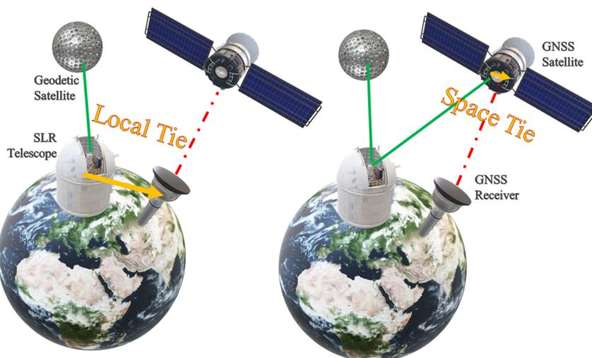
Fig. 1. SLR-GNSS co-location in space onboard GNSS satellites, after Bury et al. (2021a)
