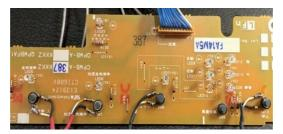
Fig. 7. Connecting the air purifier control board switches to the Sonoff 4CH controller. Source: own
