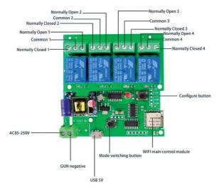
Fig. 6. Switch enabling the installation of software that integrates elements of the air purification control installation. Source: own
