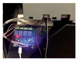
Fig. 8. Installation of the Sonoff 4CH module in an air purifier. Source: own
