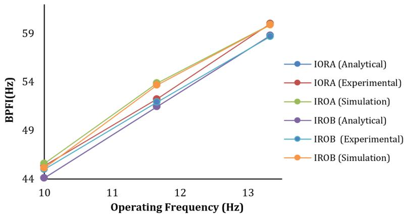
Fig. 16. Comparison of analytical, experimental and simulation BPF1 for defect at inner and outer race
