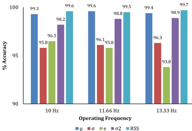
Fig. 13. Accuracy of fault prediction from extracted features using PCA
