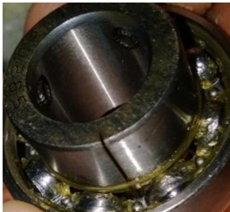
Fig. 3. 0.5 mm fault at inner race
