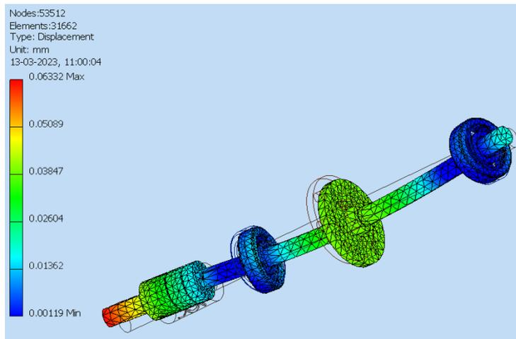
Fig. 8. Meshed model of shaft bearing system
