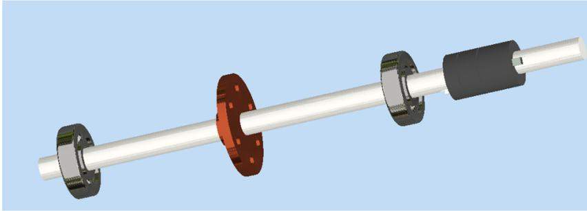
Fig. 6. CAD model of the rotor bearings arrangement
