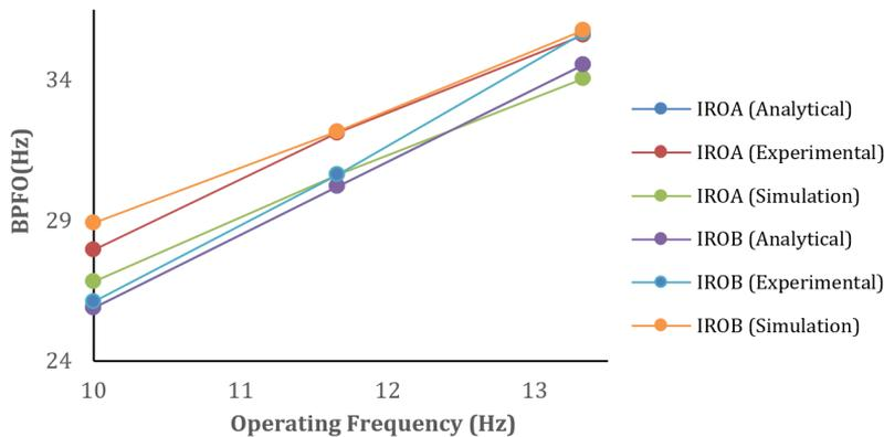
Fig. 17. Comparison of analytical, experimental and simulation BPF0 for defect at inner and outer race
