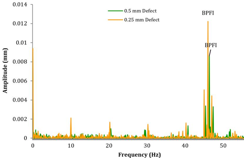
Fig. 5. Comparison of frequency spectrum of defective bearing having a fault severity of 0.25 mm and 0.5 mm at inner ring raceway for an operating speed of 600 rpm
