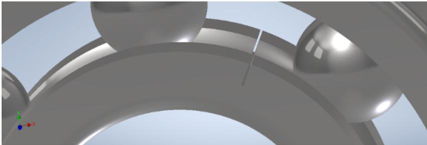
Fig. 7. 0.25 mm fault at innermost raceway
