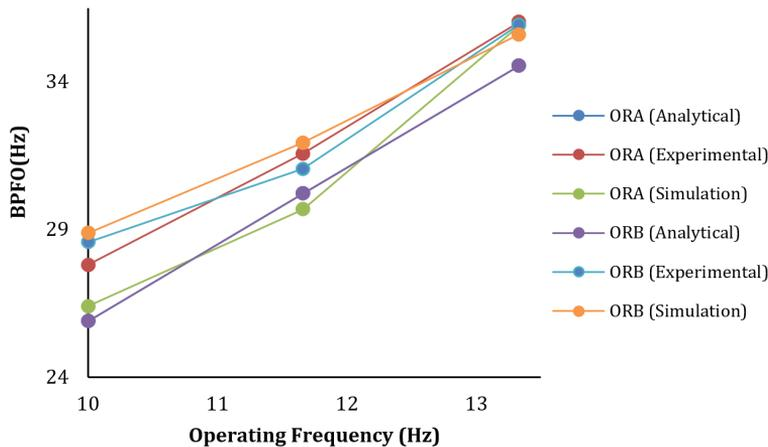
Fig. 15. Comparison of analytical, experimental and simulation BPFO for defect at outer race
