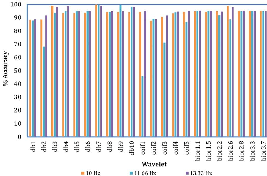
Fig. 11. Fault prediction accuracy of selected wavelets
