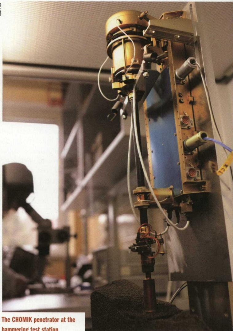
**The CHOMIK penetrator at the hammering test station**
