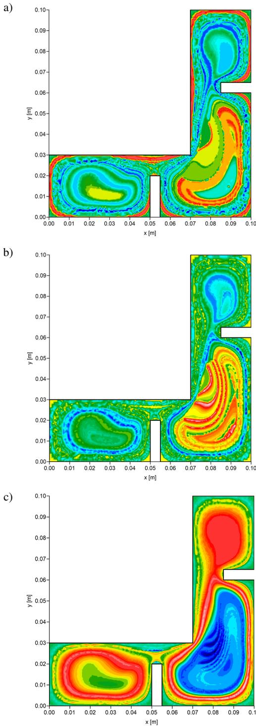
**Fig. 8.** Difference between RNN models of 2000 and 50 epochs: a) sum of ferrite and pearlite, b) bainite, c) martensite
