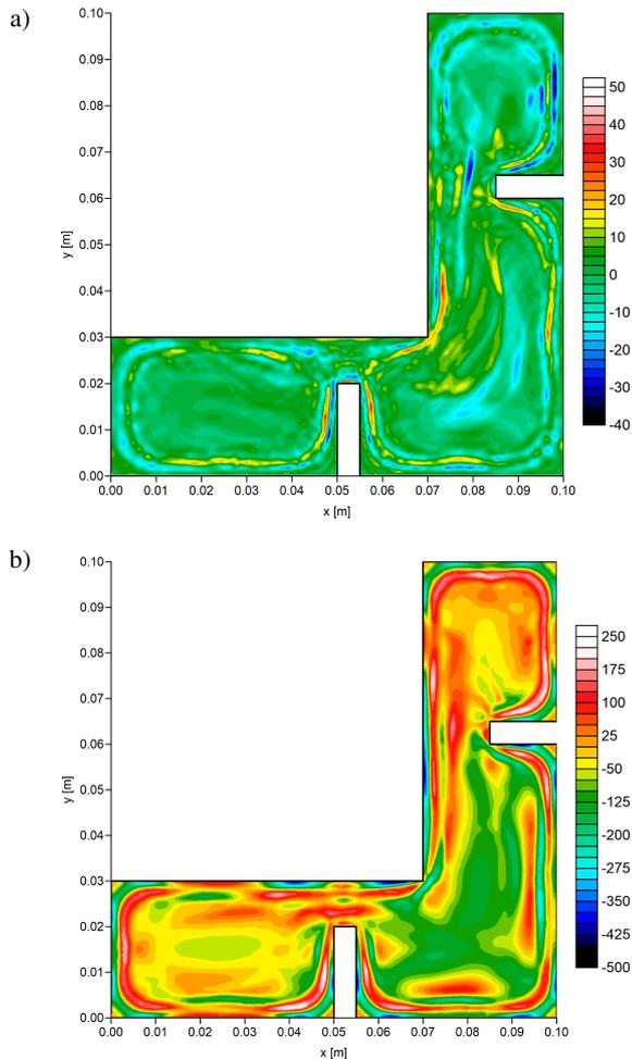
**Fig. 10.** Residual effective stresses distribution [MPa]: a) difference between RNN models, b) difference between numerical model and RNN models with 2000 epochs
