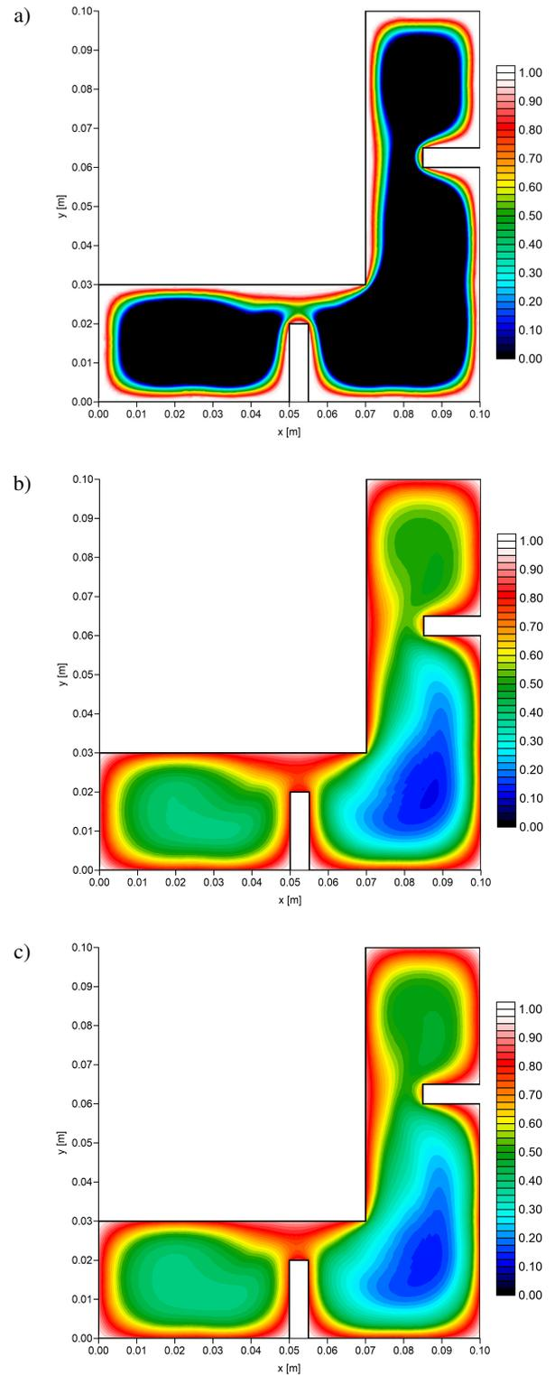
**Fig. 7.** Martensite fraction (after cooling process): a) numerical model, b) RNN 2000 epochs, c) RNN 50 epochs
