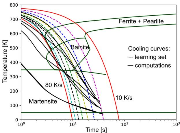
Fig. 3. CCT diagram with cooling curves
